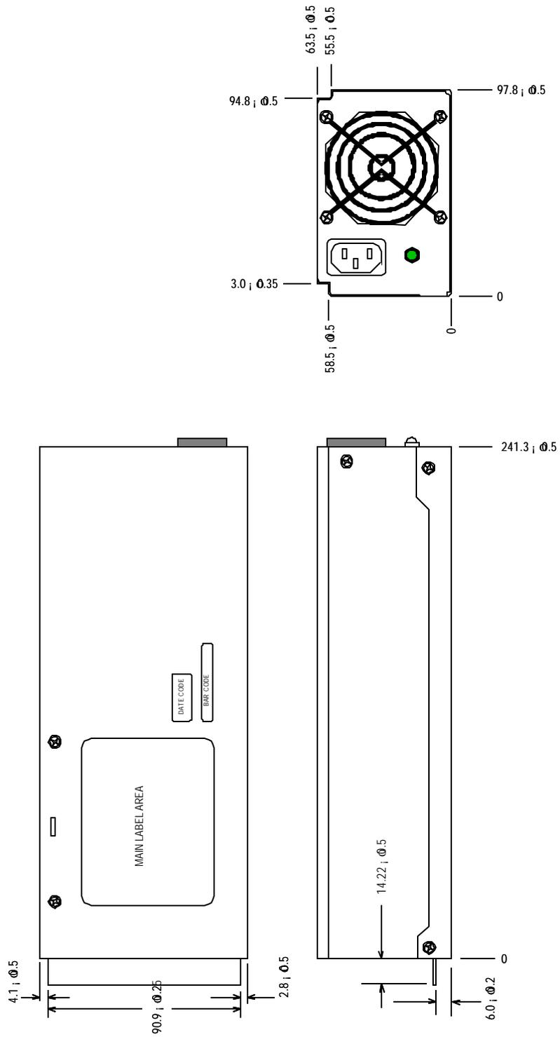
Figure 2-3. Outline Drawing Power System Enclosure
