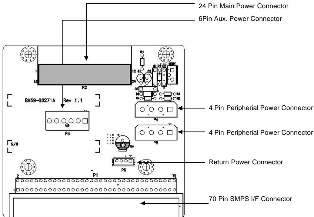
Figure 2-1. Power Distribution Board Connector Description
