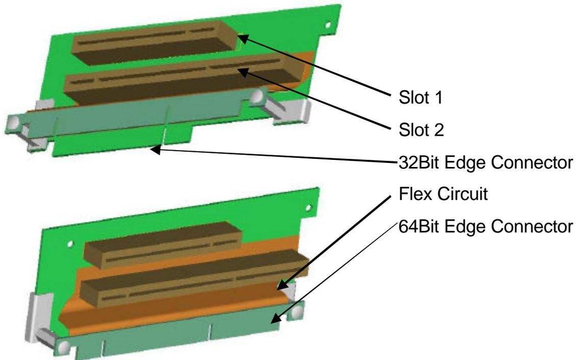
*Figure 7-2. PCI Riser for STL2 Component and Connector Description*
