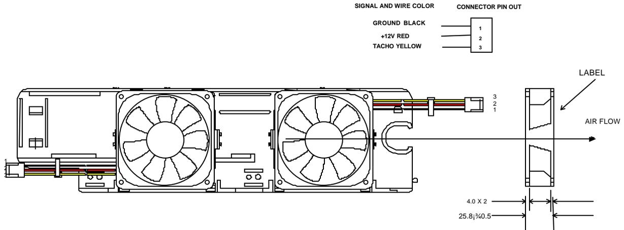
**Figure 3-1. 80mm Mid System Fan**
