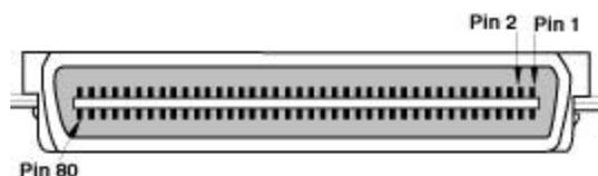
Figure 6-4. 80 Pin SCA2 Connector
