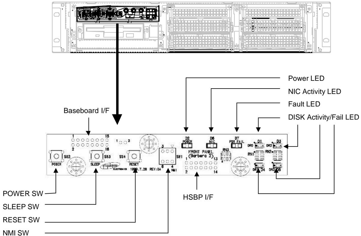
Figure 5-1. Front Panel and Functions
