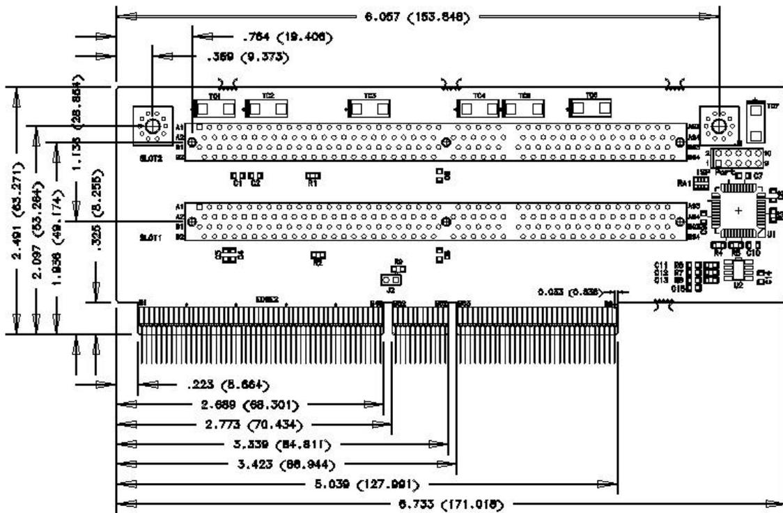
Figure 7-1. PCI Riser for L440GX+ Component and Connector Placement
