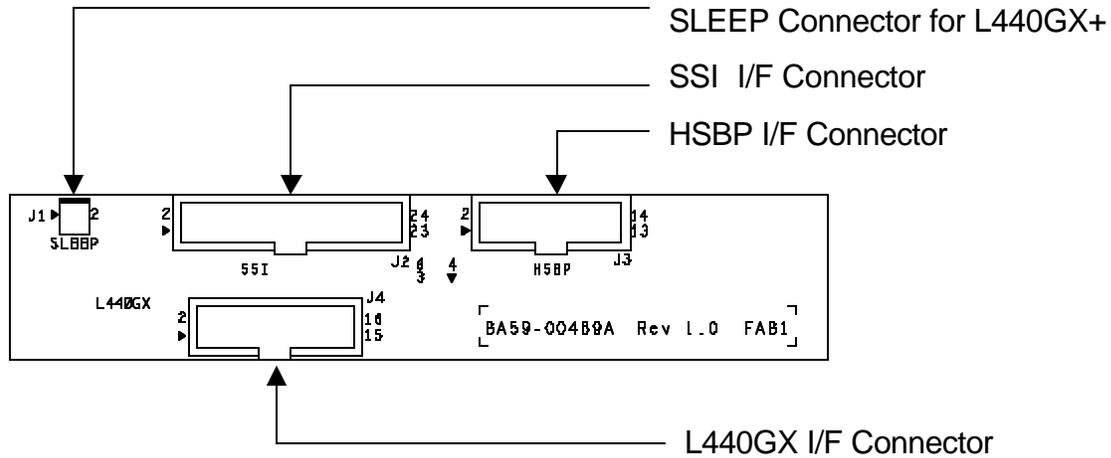
Figure 5-2. Connectors in Front Panel
