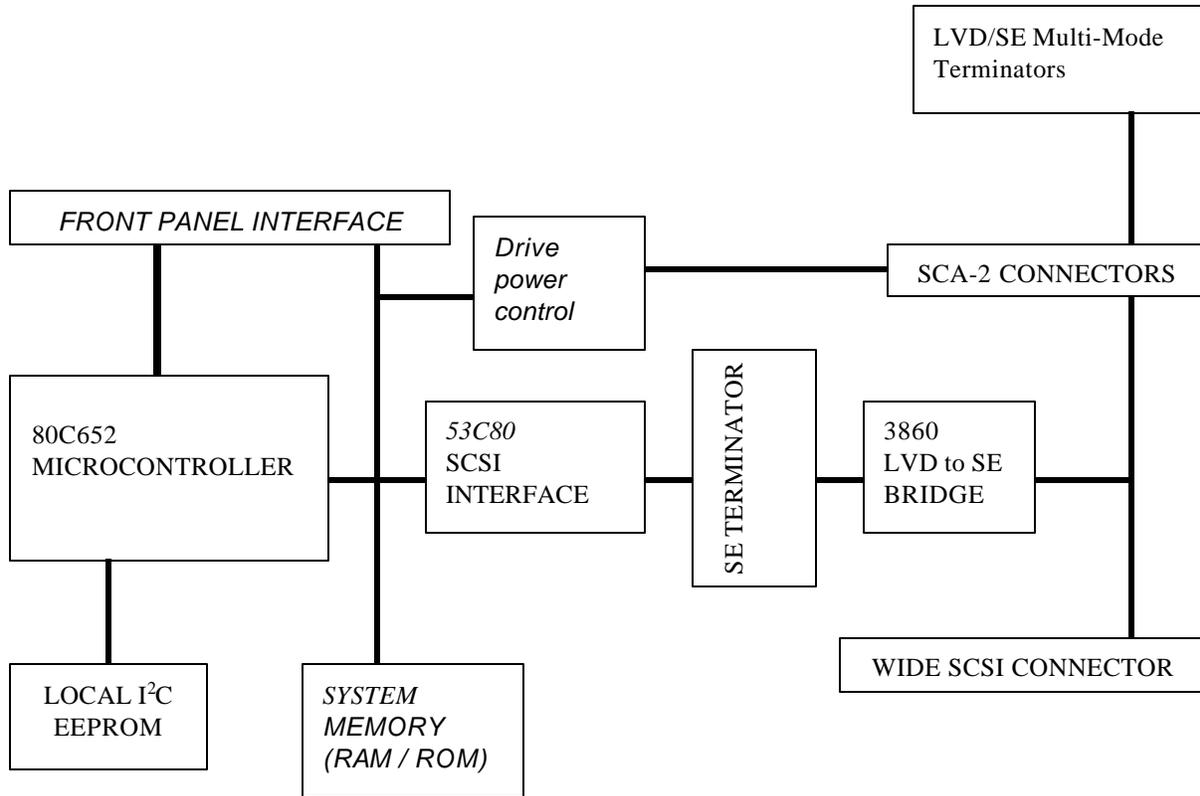
Figure 6-2. HSBP Functional Block Diagram
