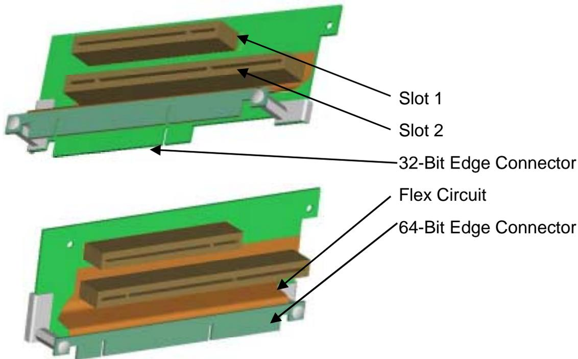
*Figure 17. PCI Riser for STL2 Component and Connector Description*
