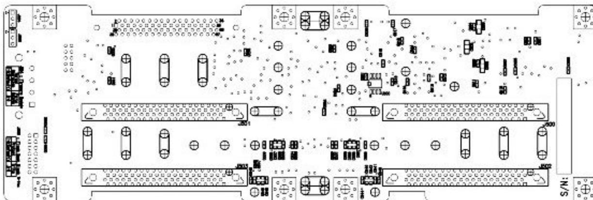
Figure 13. Hot-Swap SCSI Backplane – SCA2 Connector Side
