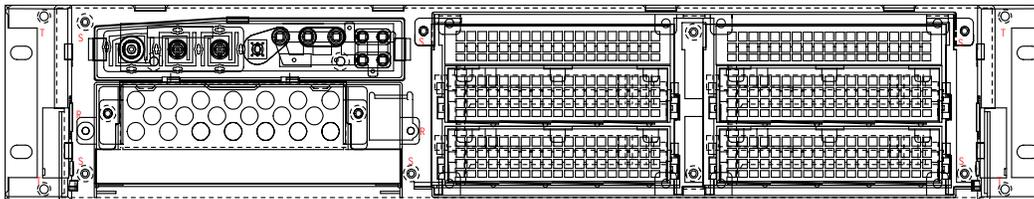
*Figure 3. Front Chassis View, without Bezel*
