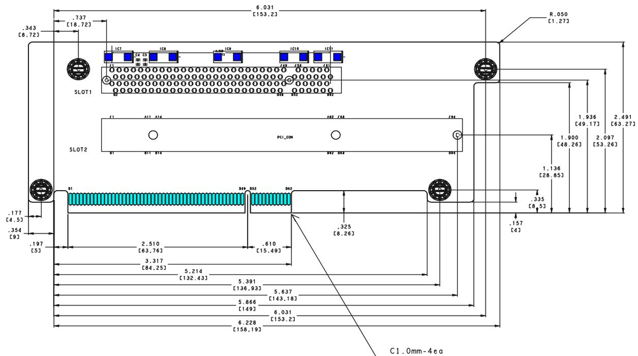
Figure 18. Component and Connector Placement of Rigid Printed Circuit
