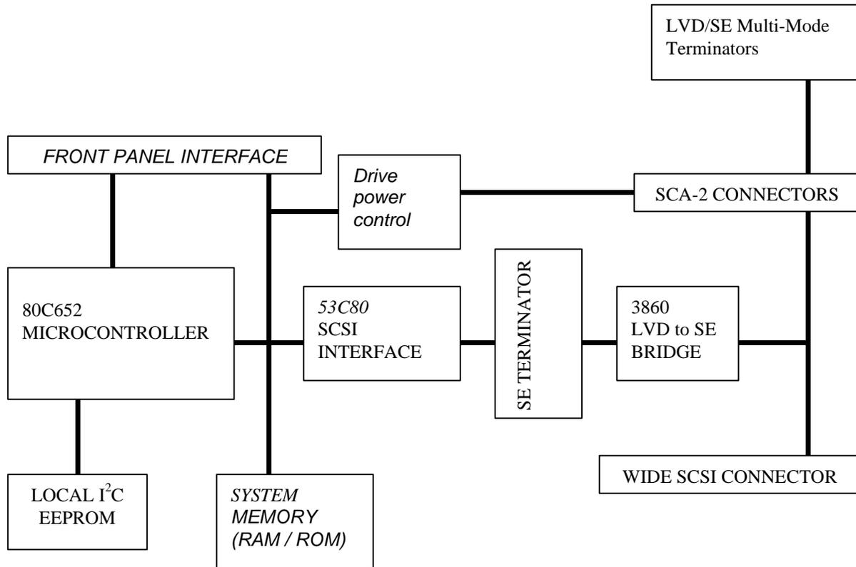
Figure 14. HSBP Functional Block Diagram
