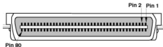
Figure 15. 80-Pin SCA2 Connector
