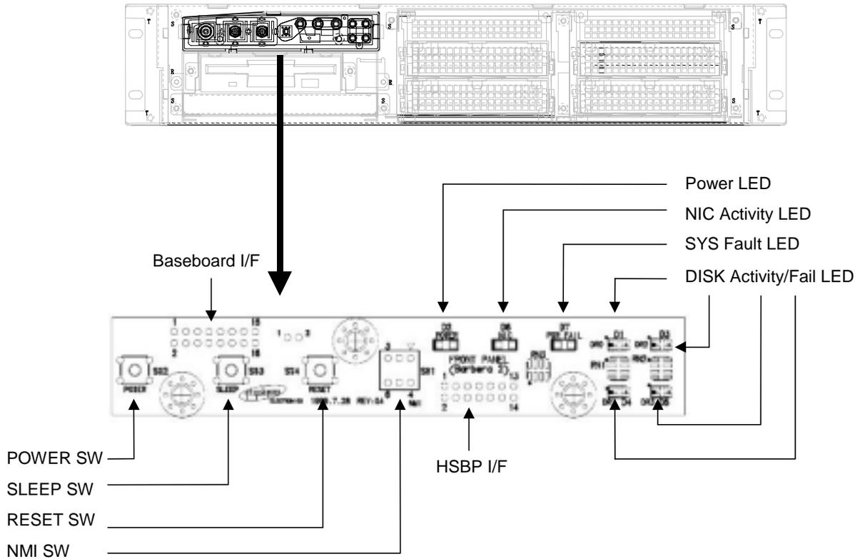
Figure 10. Front Panel and Functions
