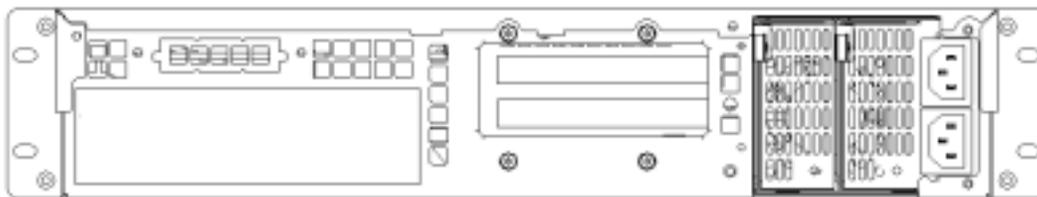
*Figure 4. Rear Chassis View (1+1 Redundant Configuration)*
