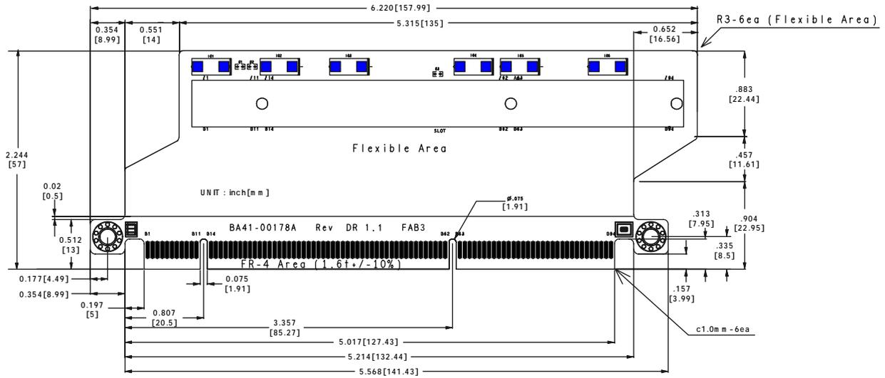
Figure 19. Component and Connector Placement of Flexible Printed Circuit
