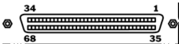
Figure 16. 68-Pin SCSI Cable Connector
