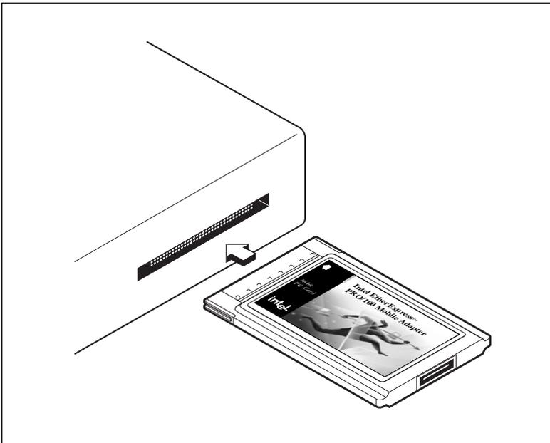
Inserting the PRO/100 PC Card into the Computer
