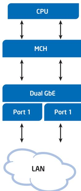
**Figure 1.** Network data flow in a previous-generation platform
