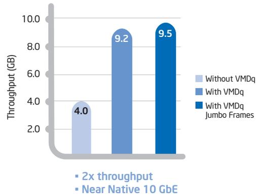
**Figure 6.** Tests measure wire speed Receive (Rx) side performance with VMDq on Intel® 82598 10 Gigabit Ethernet Controllers.
