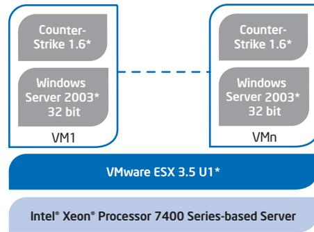
Figure 14. Test software stack.
