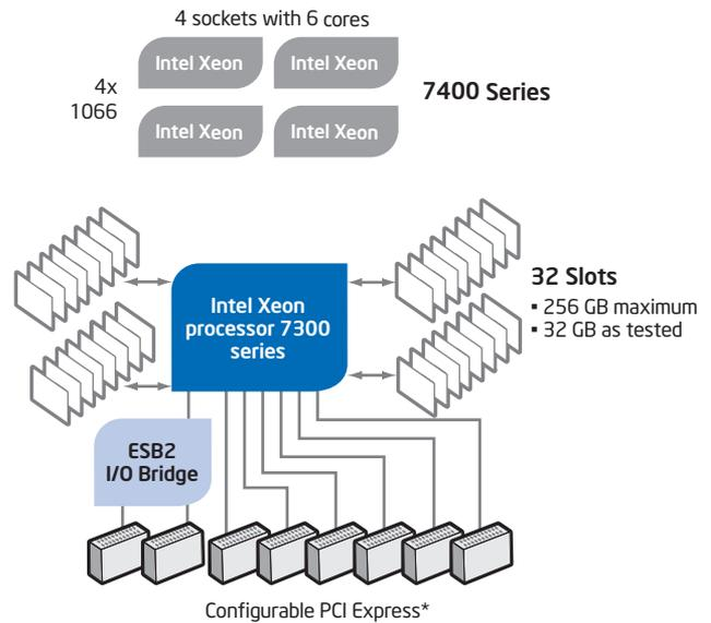
Figure 2. Intel® Xeon® processor 7300 platform high-level architecture.
