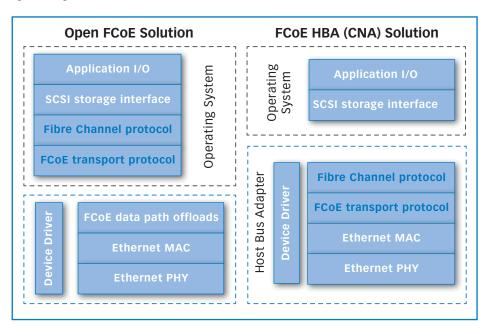
**Figure 2.** Overview of Fibre Channel over Ethernet (FCoE) host bus adapters (converged network adapters) and Open FCoE initiator solutions
