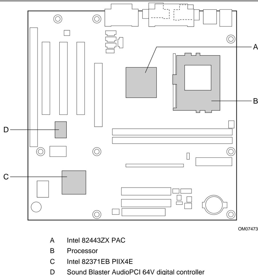
**Figure 13. Thermally-sensitive Components**
