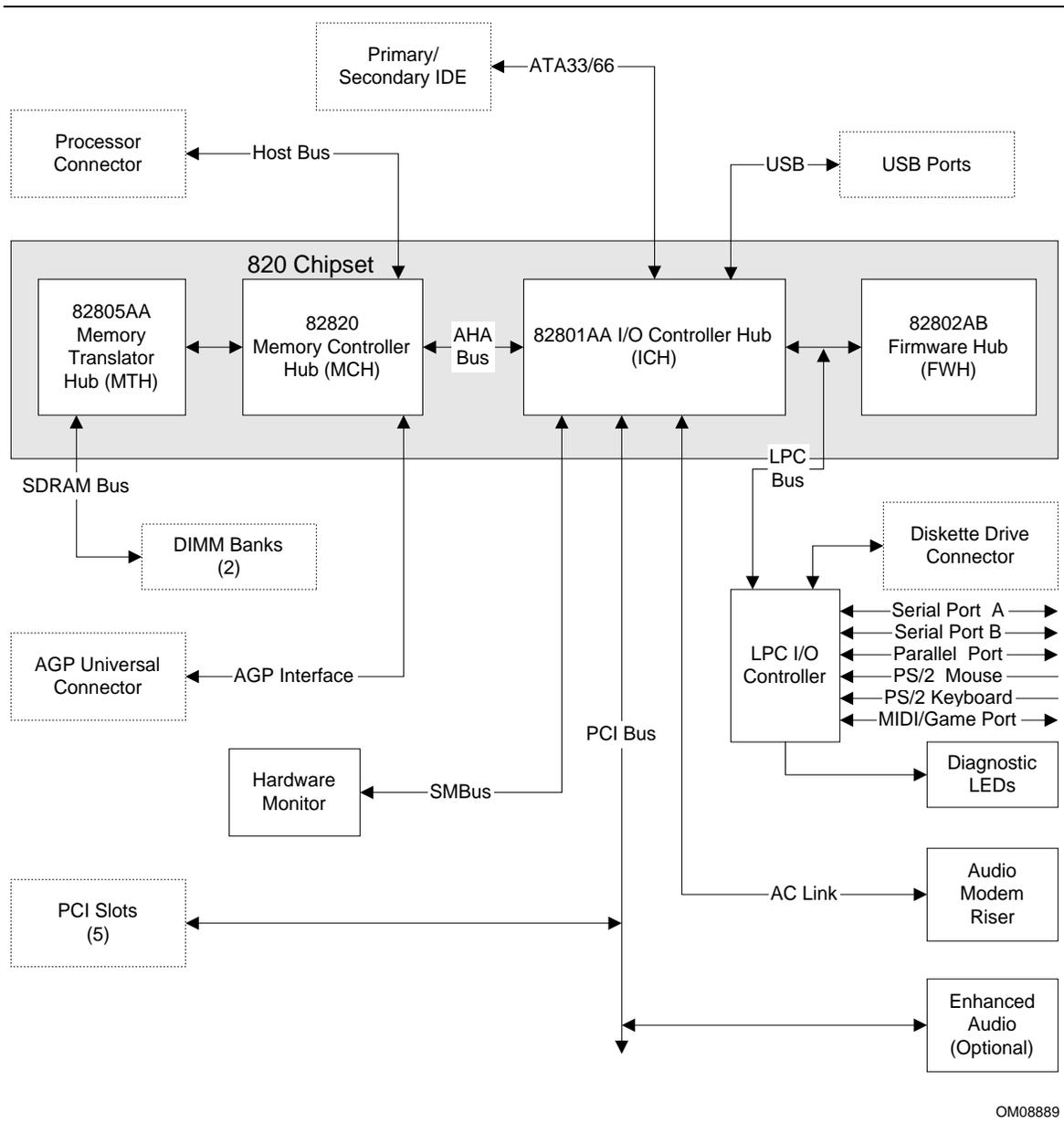
Figure 2. Block Diagram
