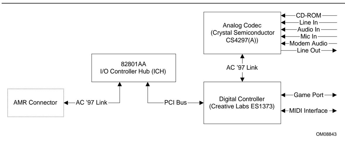
**Figure 4. Block Diagram of AC '97 V 1.03 Compatible Audio Subsystem with Creative Labs ES1373 Controller and AMR Connector**
