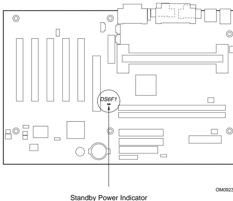
**Figure 6. Location of Standby Power Indicator LED**
