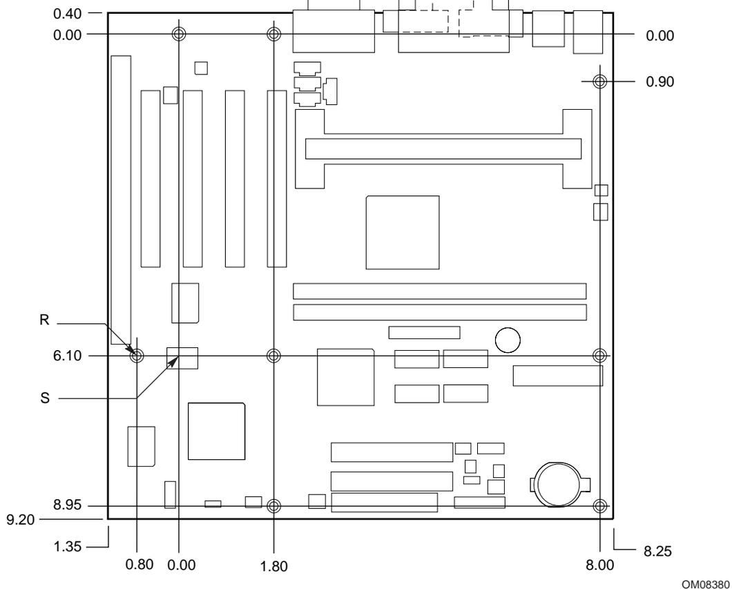
**Figure 11. microATX Motherboard Dimensions**
