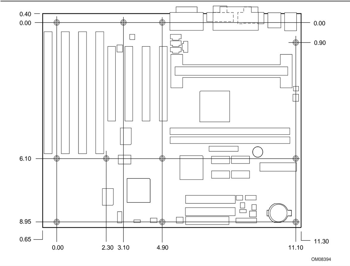
**Figure 12. Full ATX Motherboard Dimensions**
