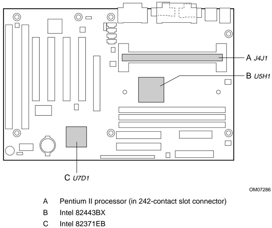
**Figure 10. Thermally-Sensitive Components**
