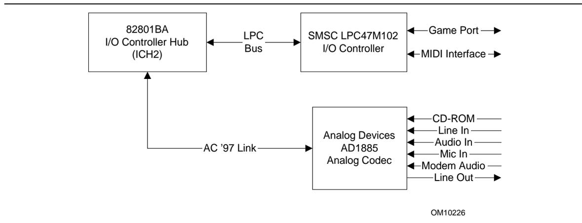
**Figure 4. Block Diagram of Basic Audio Subsystem**
