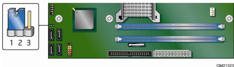
**Figure 24. Location of the BIOS Configuration Jumper Block**
