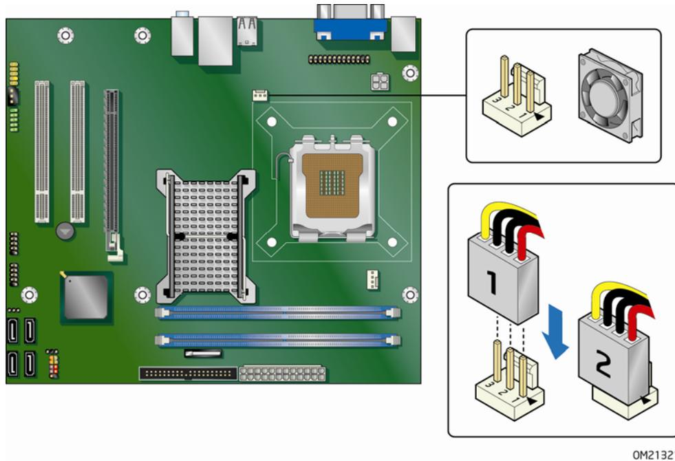
Figure 22. Location of the Rear Chassis Fan Header
