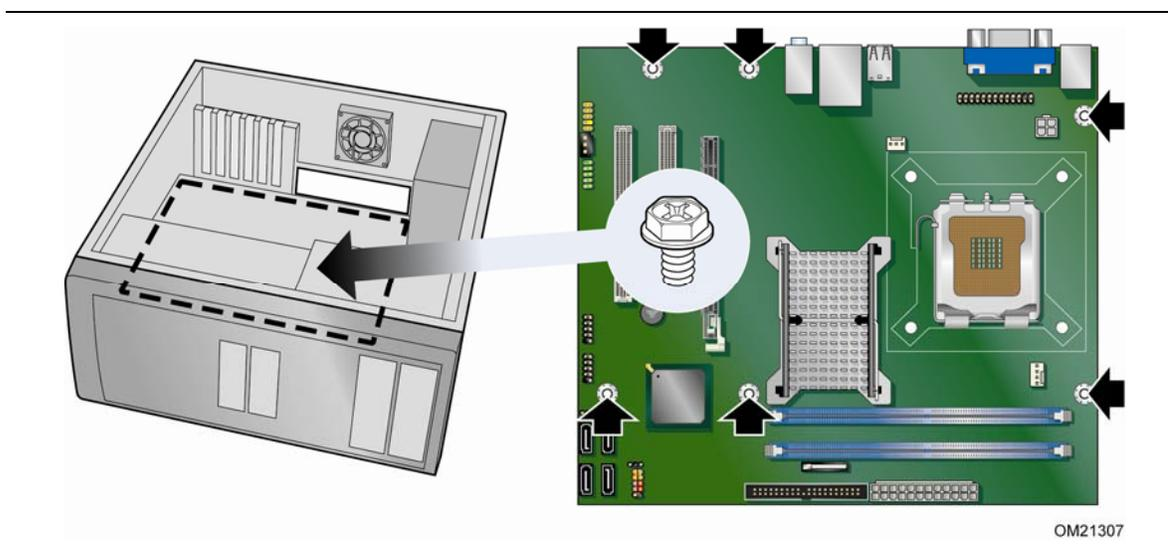
**Figure 5. Intel Desktop Board DG41RQ Mounting Screw Hole Locations**
