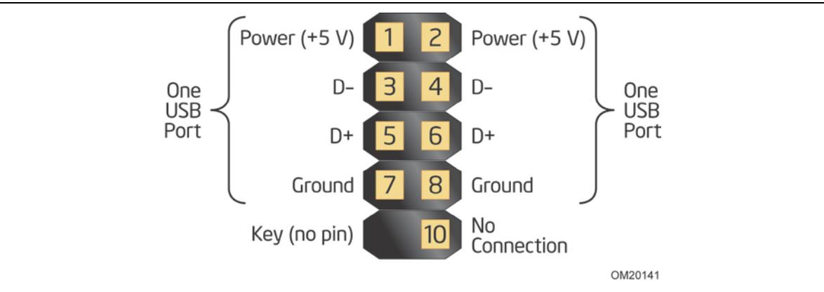
**Figure 13. Connection Diagram for Front Panel USB Header**
