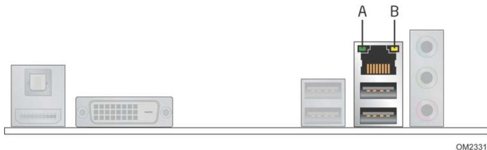
**Figure 4. LAN Connector LED Locations**
