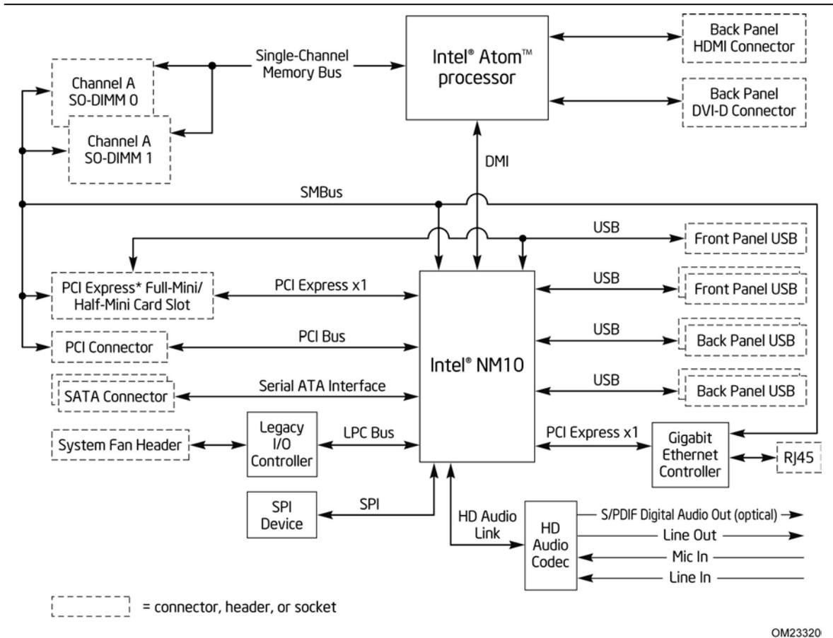
Figure 2. Block Diagram
