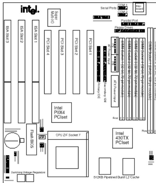
**Figure 1. Motherboard Components**
