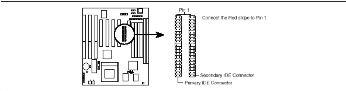
**Figure 7. PCI IDE Connectors**
