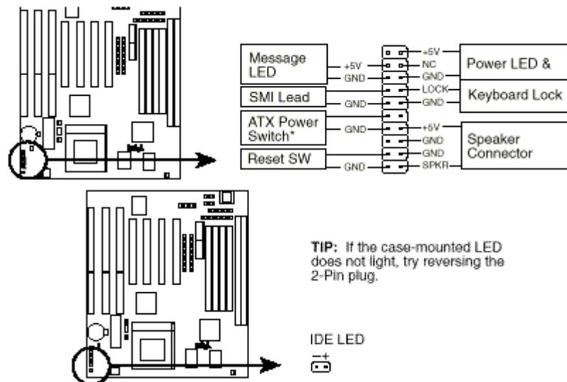
Figure10. Front Panel I/O Connectors
