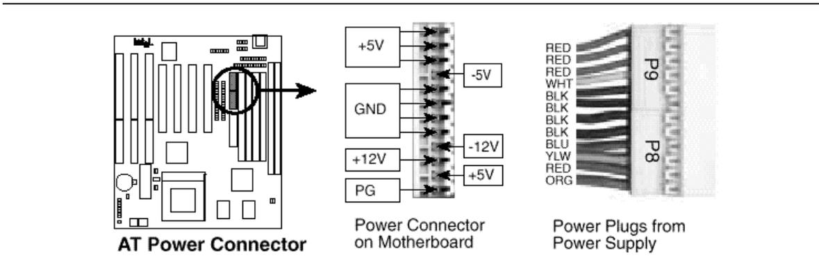
**Figure 8. AT Power Connector**
