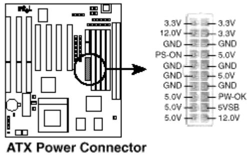
Figure 9. ATX Power Connector
