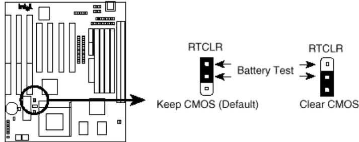
Figure 14. RTC, RTCLR Jumper
