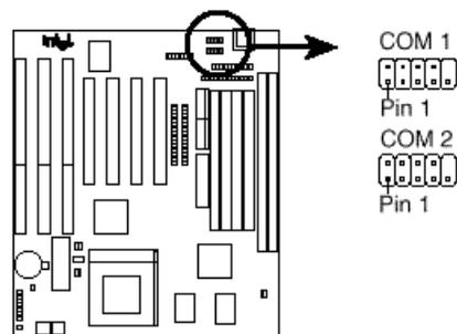
Figure 3. Serial Port Headers
