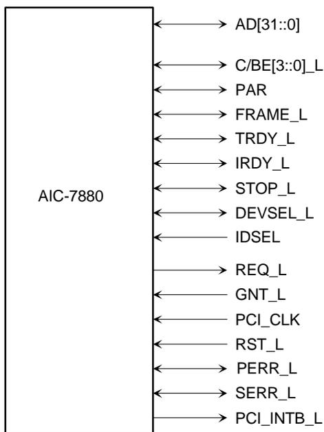
Figure 2-10 Embedded SCSI PCI Signals
