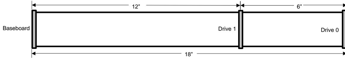
Figure 2-6 IDE Cable Requirements
