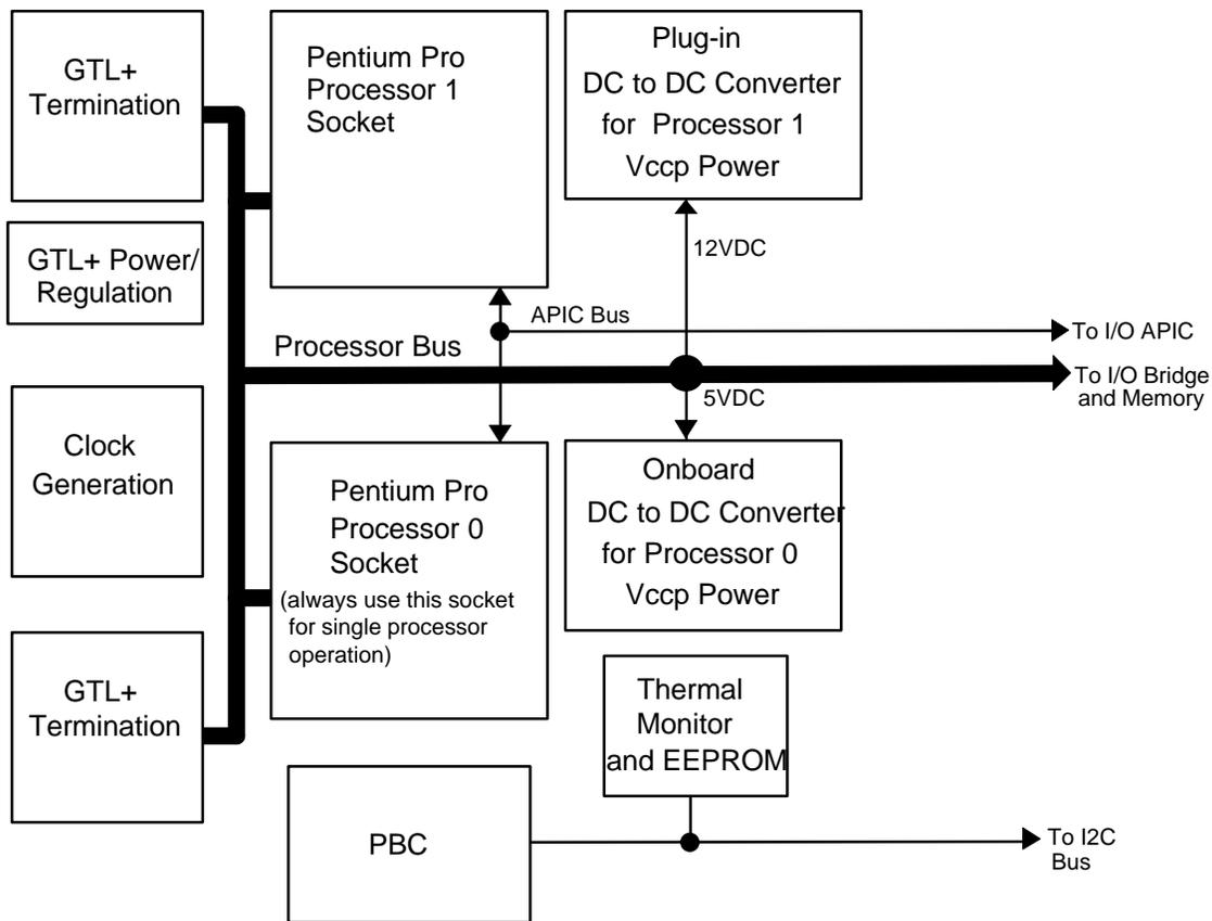
Figure 2-3 Processor Subsystem Block Diagram
