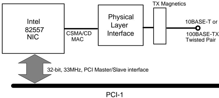
Figure 2-12 Network Controller Subsystem
