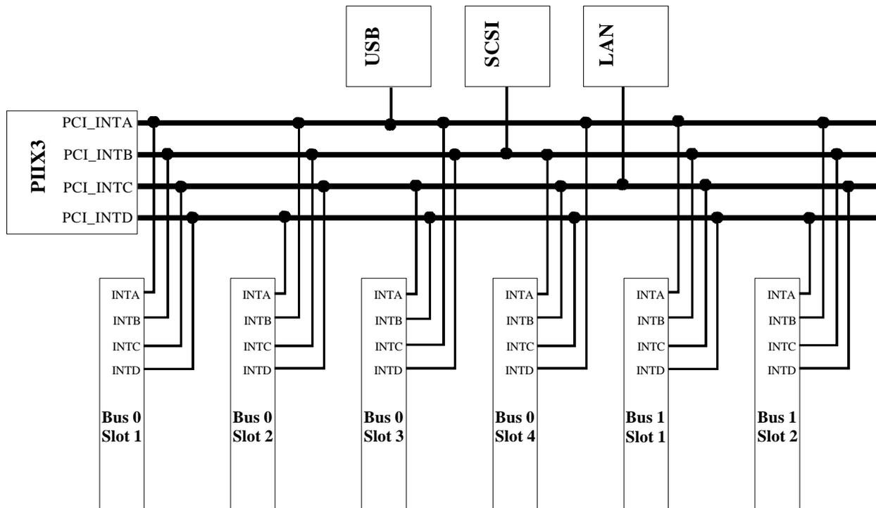
Figure 2-8 PCI Interrupt Routing
