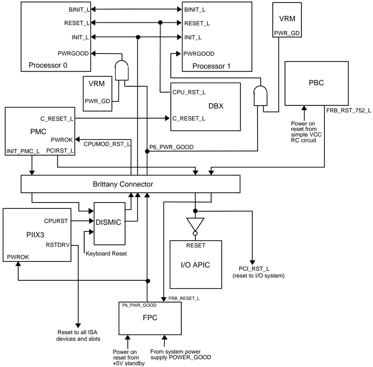
Figure 2-16 System Reset Flow
