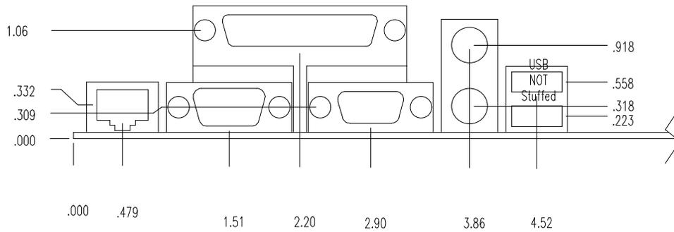
Figure 6-4 I/O Connector Mechanical Diagram
