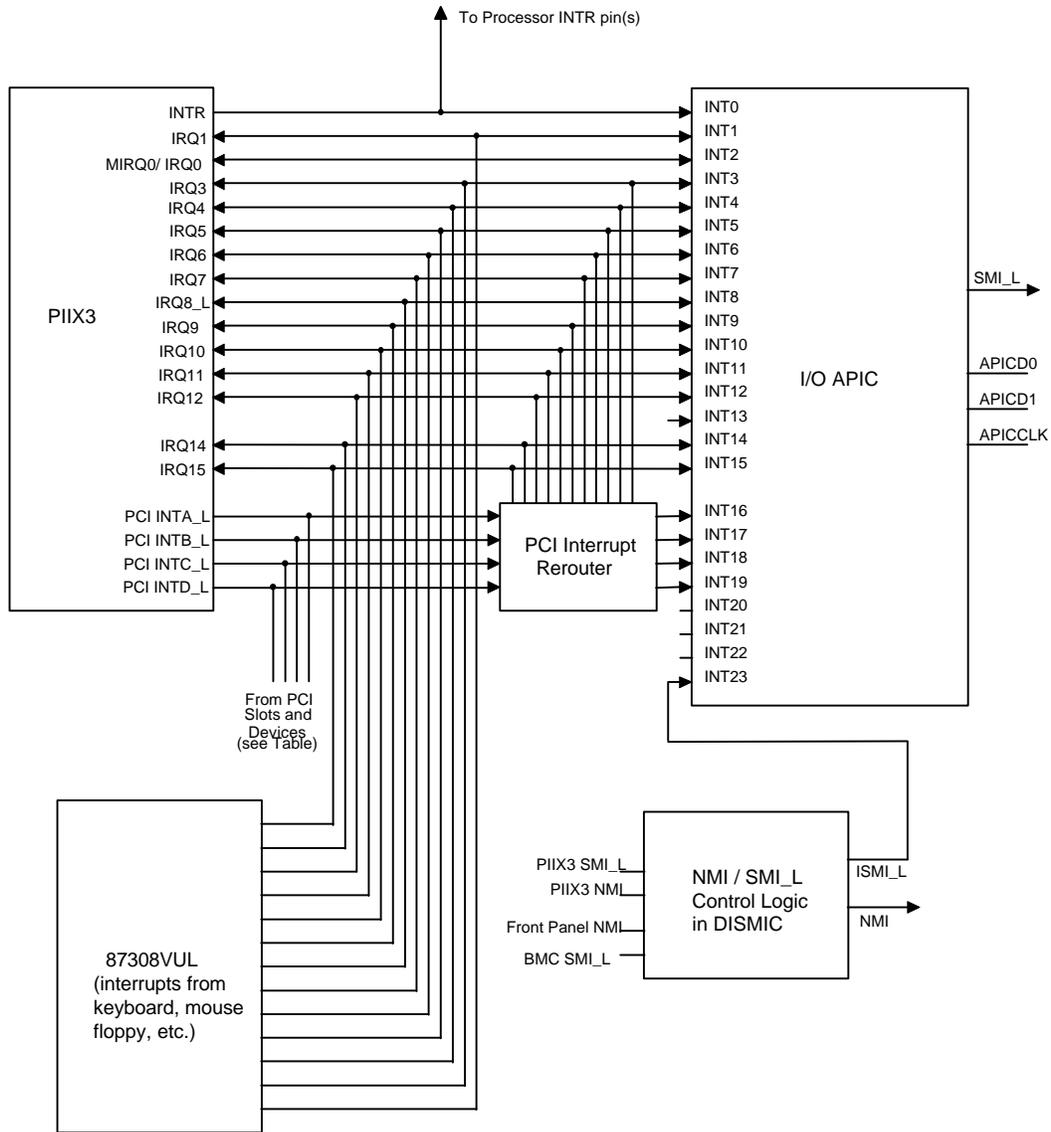
Figure 2-9 Interrupt Connections
