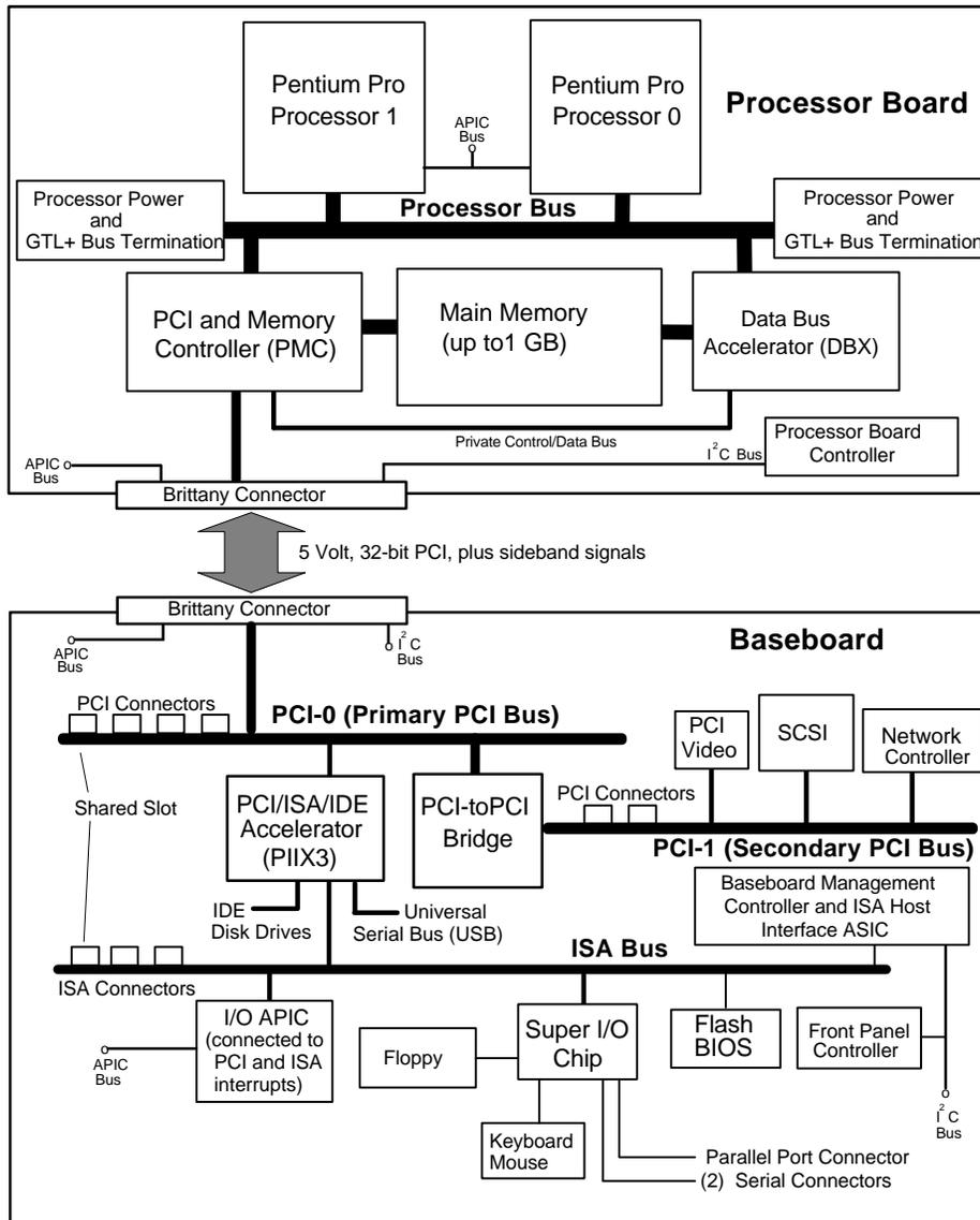
Figure 2-1 B440FX DP Server Functional Block Architecture
