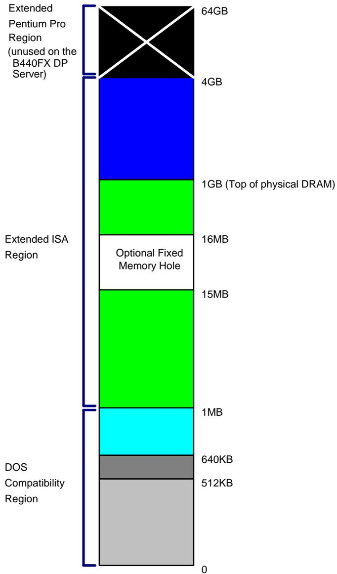
Figure 3-3 Pentium Pro Processor Memory Address Space
