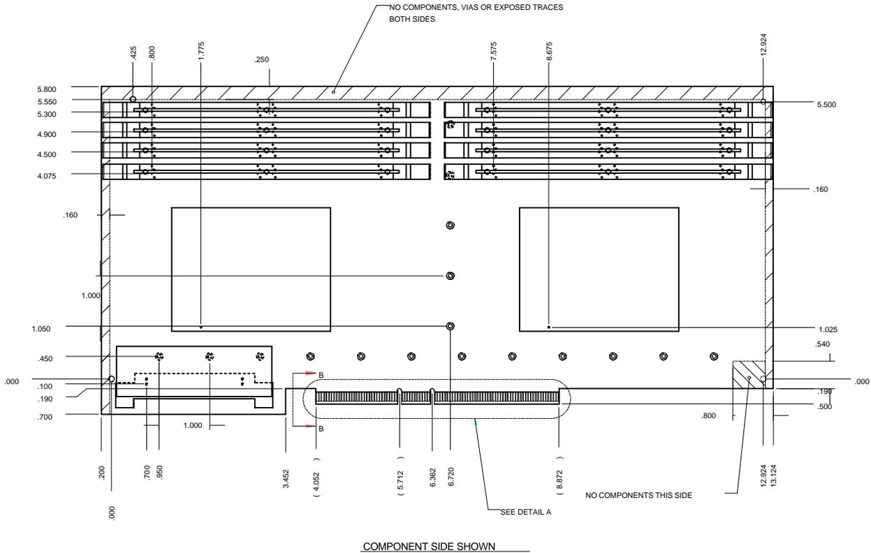
Figure 6-1 Processor Board Mechanical Diagram
