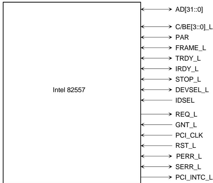
Figure 2-13 Embedded NIC PCI Signals
