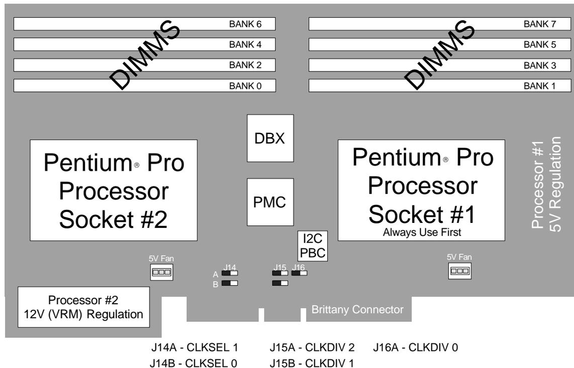
Figure 2-2 B440FX DP Server Processor Board Layout
