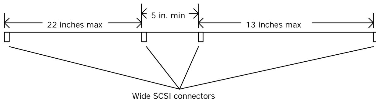
Figure 12. Single-Ended SCSI Bus Cable Length Specifications
