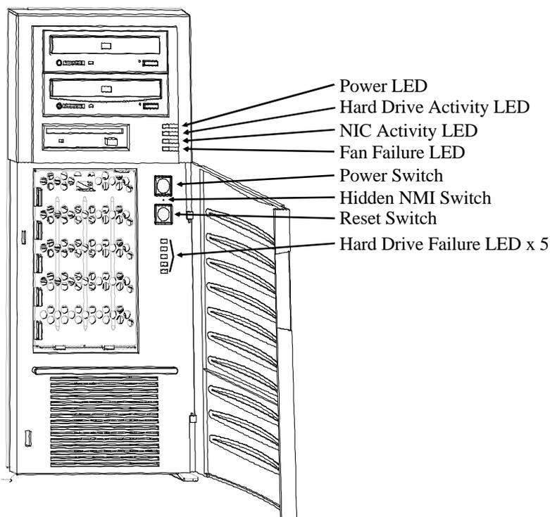
Figure 10: Front Panel and Functions
