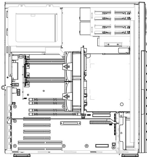
Figure 5: Side View showing N440BX DP Server board
