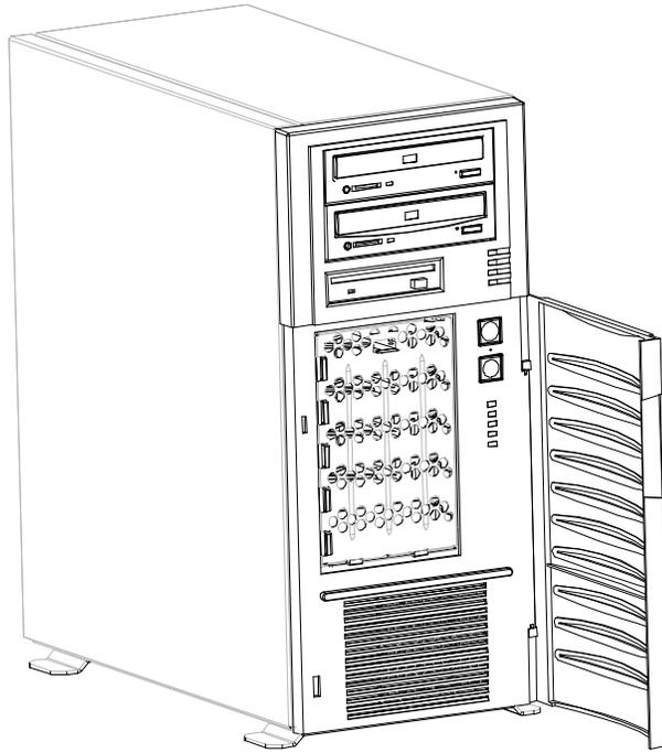
Figure 3: Front Isometric View, open Drive Access Door
