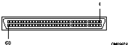
Figure 14: 68 pin SCSI wide connector
