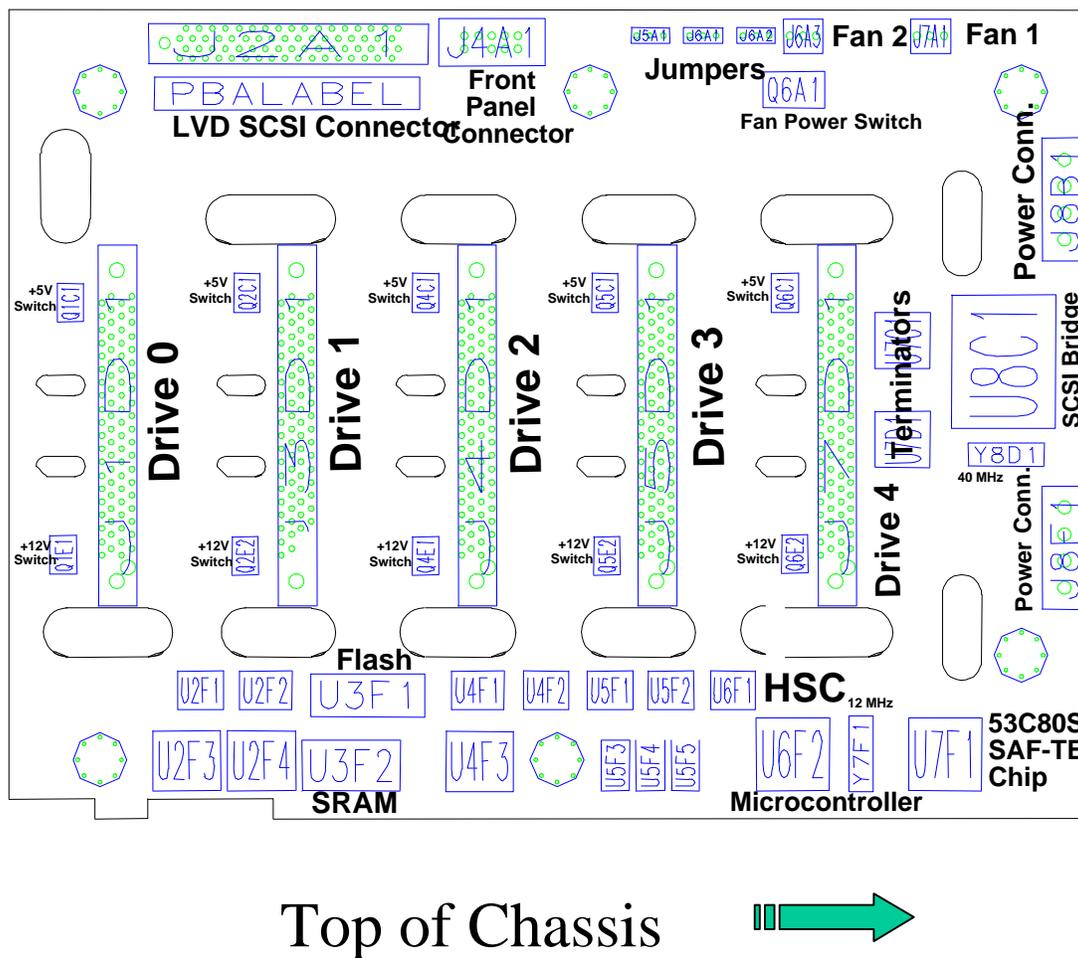
Figure 11. Astor II Hot-Swap SCSI Backplane Component and Connector Placement
