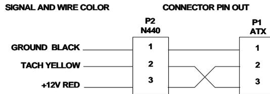
Figure 18: System Fan pinouts
