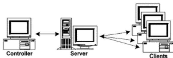
For benchmark purposes on the L440GX+, Microsoft\* Windows NT 4.0 was used as the primary test operating system. ServerBench 4.02 was used running the standard test file, "sys60.tst". No modifications to the standard test suite were made.
