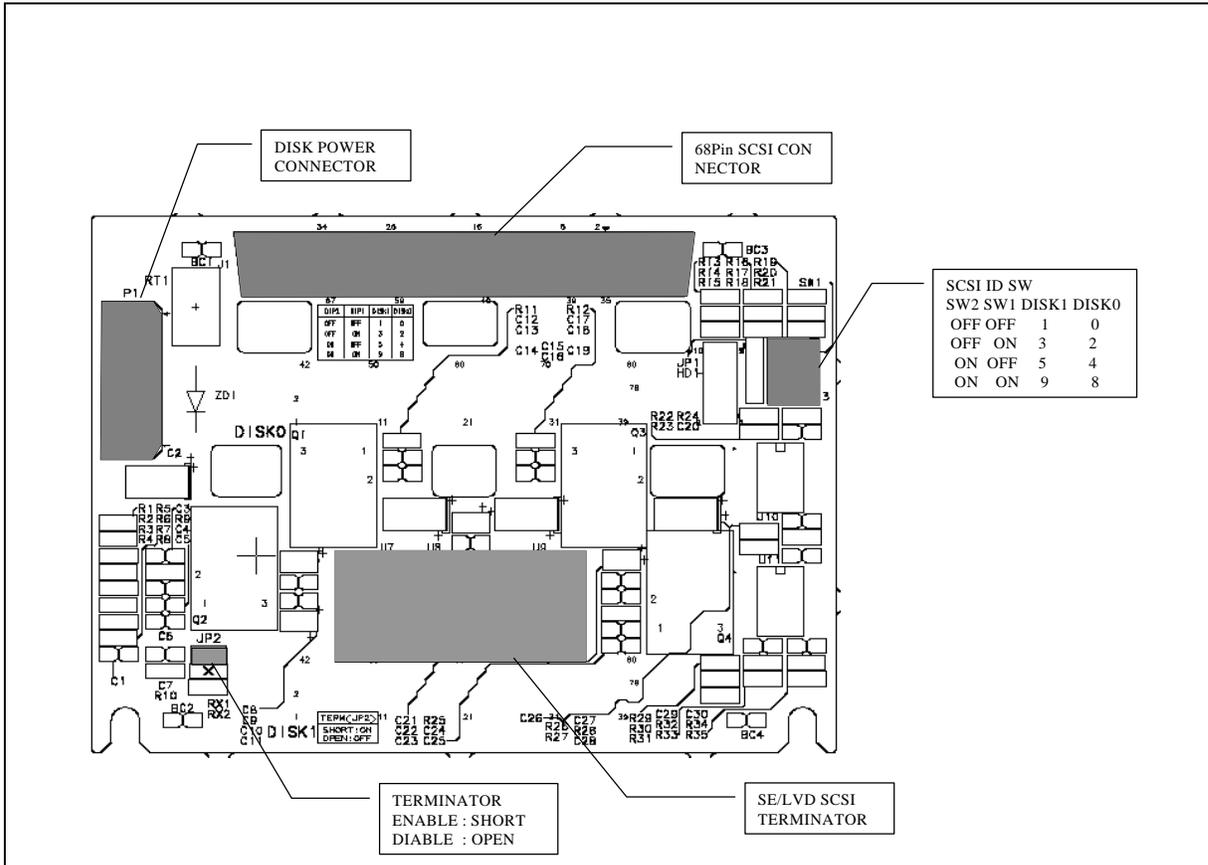
Figure 6. Functional Diagram of the Hot-Swap SCSI Backplane
