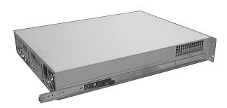
Locate the front and rear rail brackets for one side of the rail kit. One pair (A and B) exists for each side of the cabinet rack.
