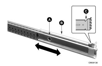
8. To attach the rear part of the rail system to the rear rail bracket (A), slide the rail system within the rail brackets such that you can place a screw through the rail's hole (B) and into the rail bracket's slot. Loosely tighten the screw and nut. You should be able to slide the entire rail system back and forth in the rail brackets. When you have centered the rails in the bracket, tighten the fastening screws and nuts.
