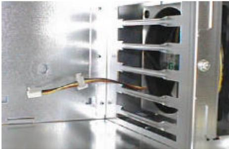
Be sure and notice that there are two connectors on the front fan in the Astor II chassis. The connector on the right is for the N440BX and the connector on the left is for the L440GX.
