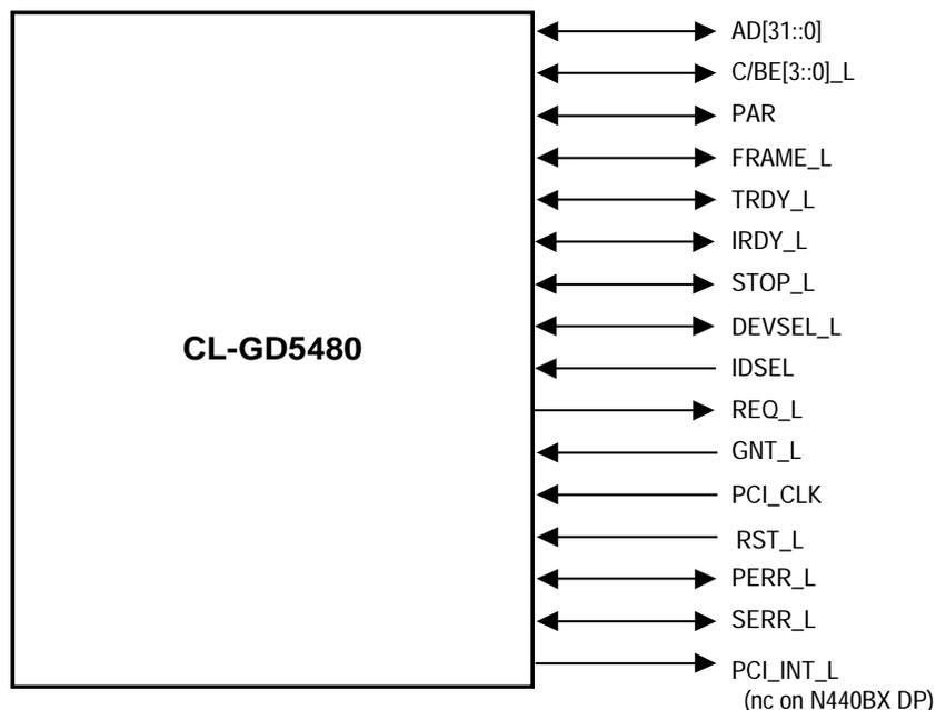
Figure 3-2. Video Controller PCI Signals
