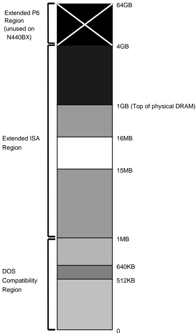
Figure 15. Pentium II/Pentium III processor memory address space
