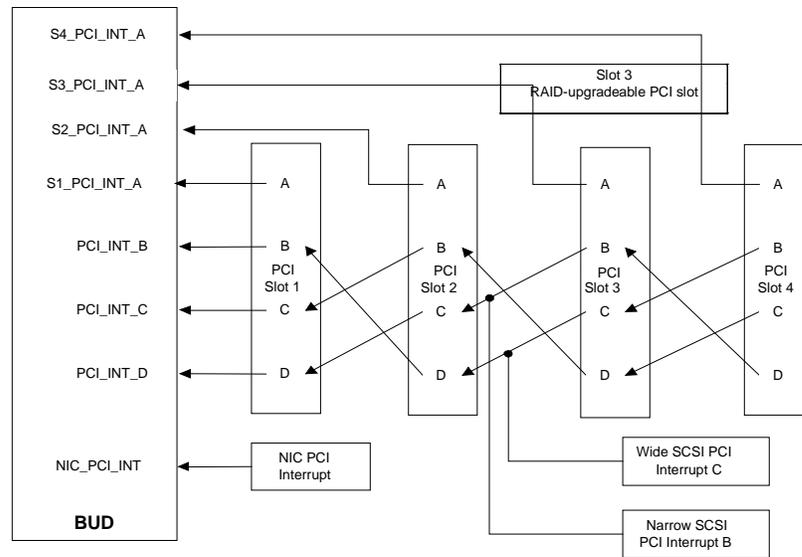
Figure 3-7. PCI Slot Interrupt Swizzle
