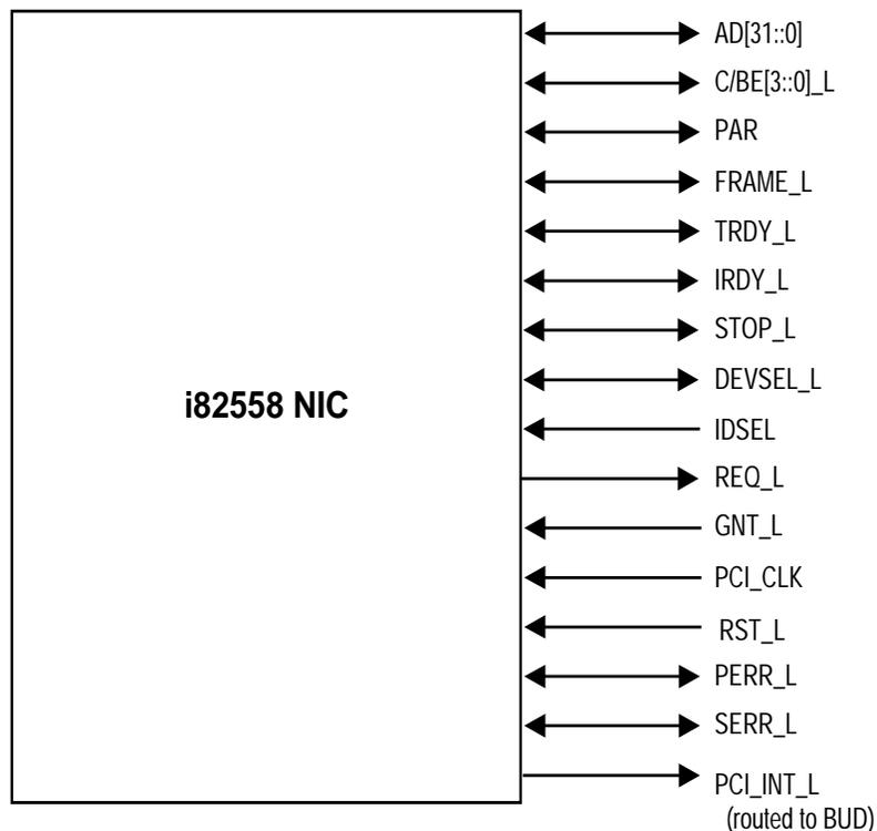
Figure 1-3. Embedded NIC PCI Signals
