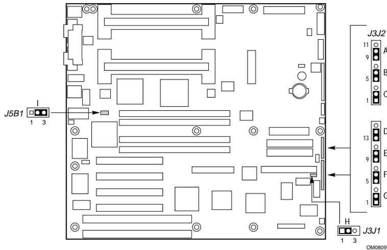
Figure 1.4 N440BX Jumper Connectors
