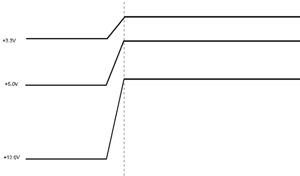
Figure 6-1. DC Voltage Sequencing
