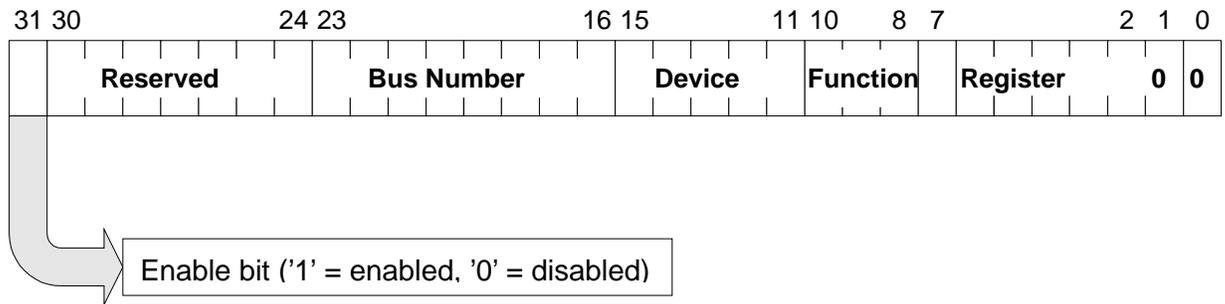
Figure 18 CONFIG\_ADDRESS Register
