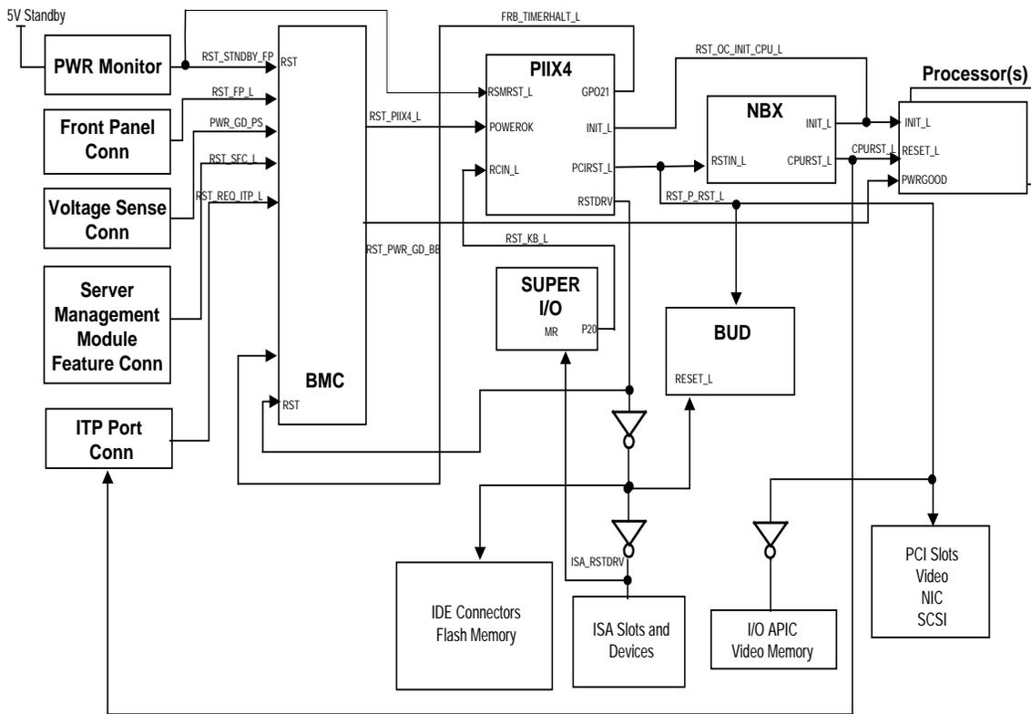
Figure 3-4. Reset Flow Diagram
