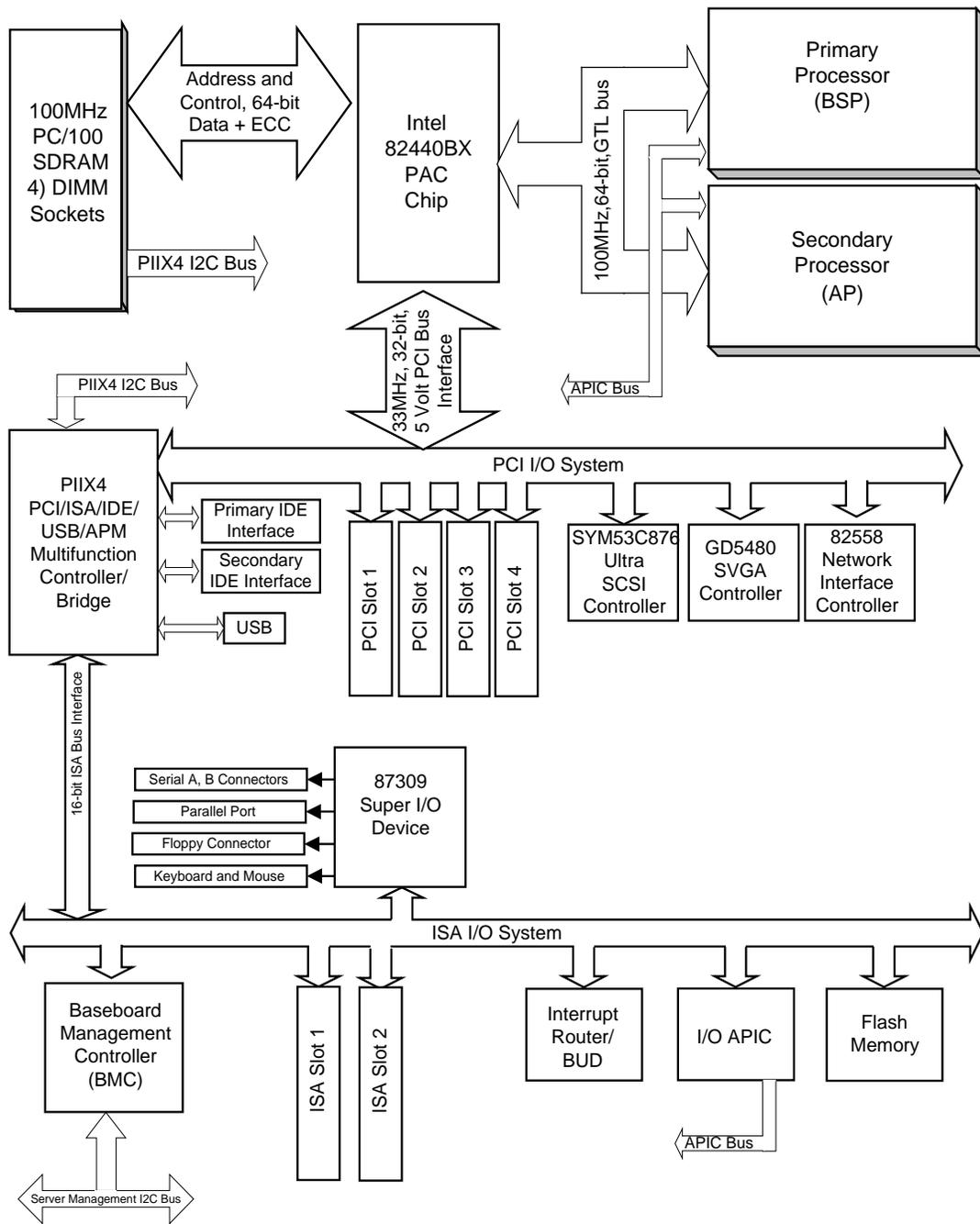
Figure 1.1 N440BX Server Functional Block Architecture
