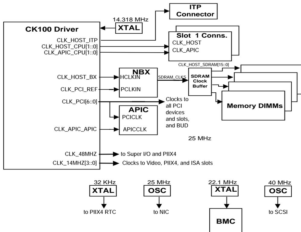
Figure 3-5. Clock Generation and Distribution
