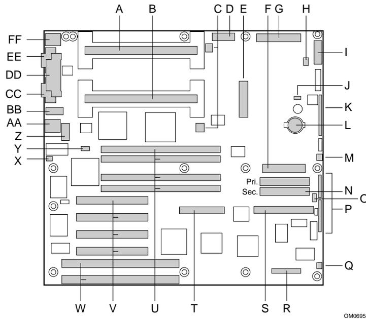
**Figure 2. Server Board Connector and Component Locations**
