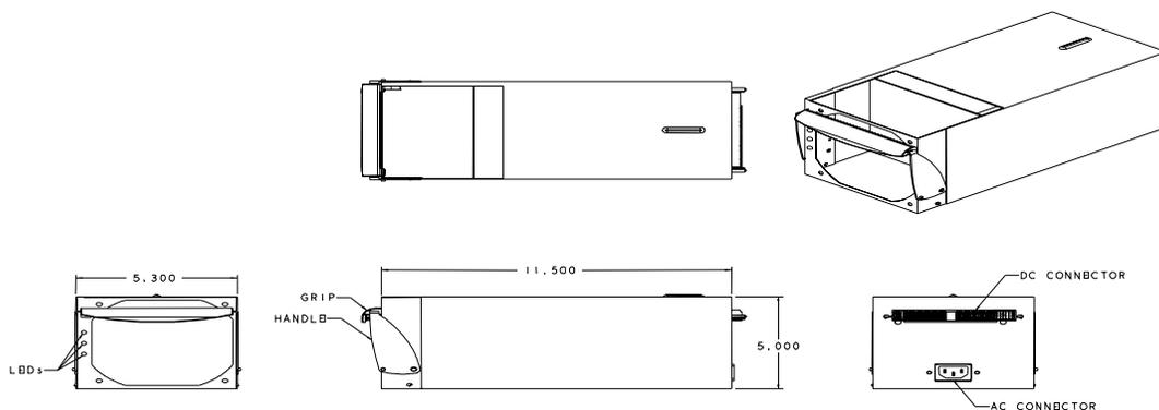
**Figure 5-1: Outline Drawing of Power Supply Enclosure**
