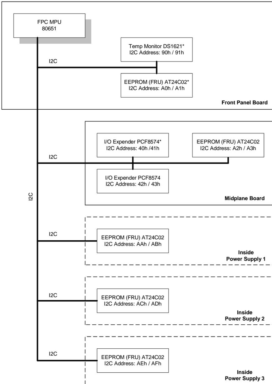
**Figure 10-2: Devices Not Supporting Multimaster Mode**
