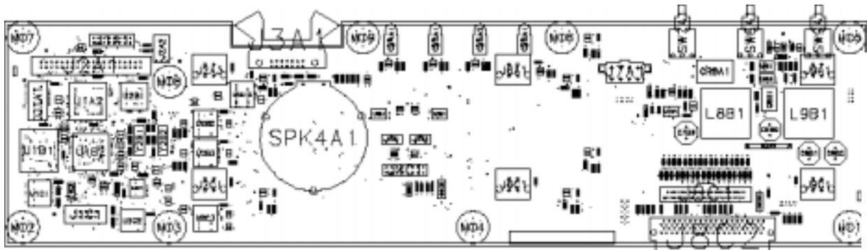
*Figure 10-1: OCPRF100 MP Server System Front Panel Layout*
