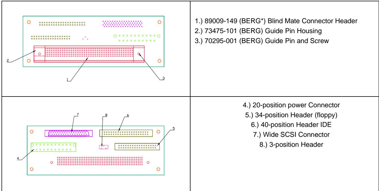
**Figure 9-1: Peripheral Bay Board (Chassis Side) Layout**
