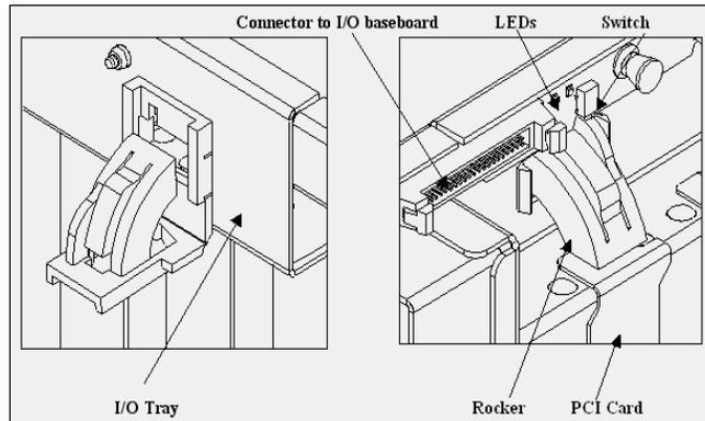
**Figure 3-9: Rocker Mechanism**
