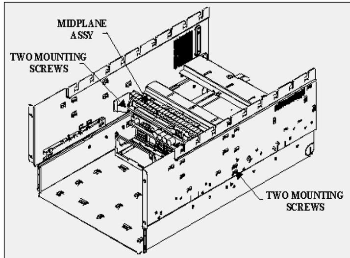
*Figure 2-11: Midplane Assembly Installed in System*
