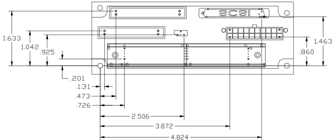
**Figure 9-2: Peripheral Bay Board (Chassis Side) Connector Layout**
