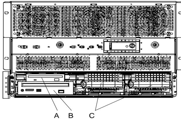
**Figure 3-7: Chassis Drive Bays**
