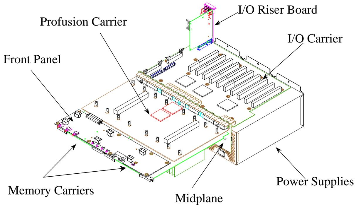
**Figure 3-2: OPRF100 Board Set/System Board Locations within Server Chassis**
