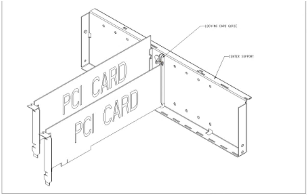
**Figure 3-10: PCI Card Retention Mechanism**
