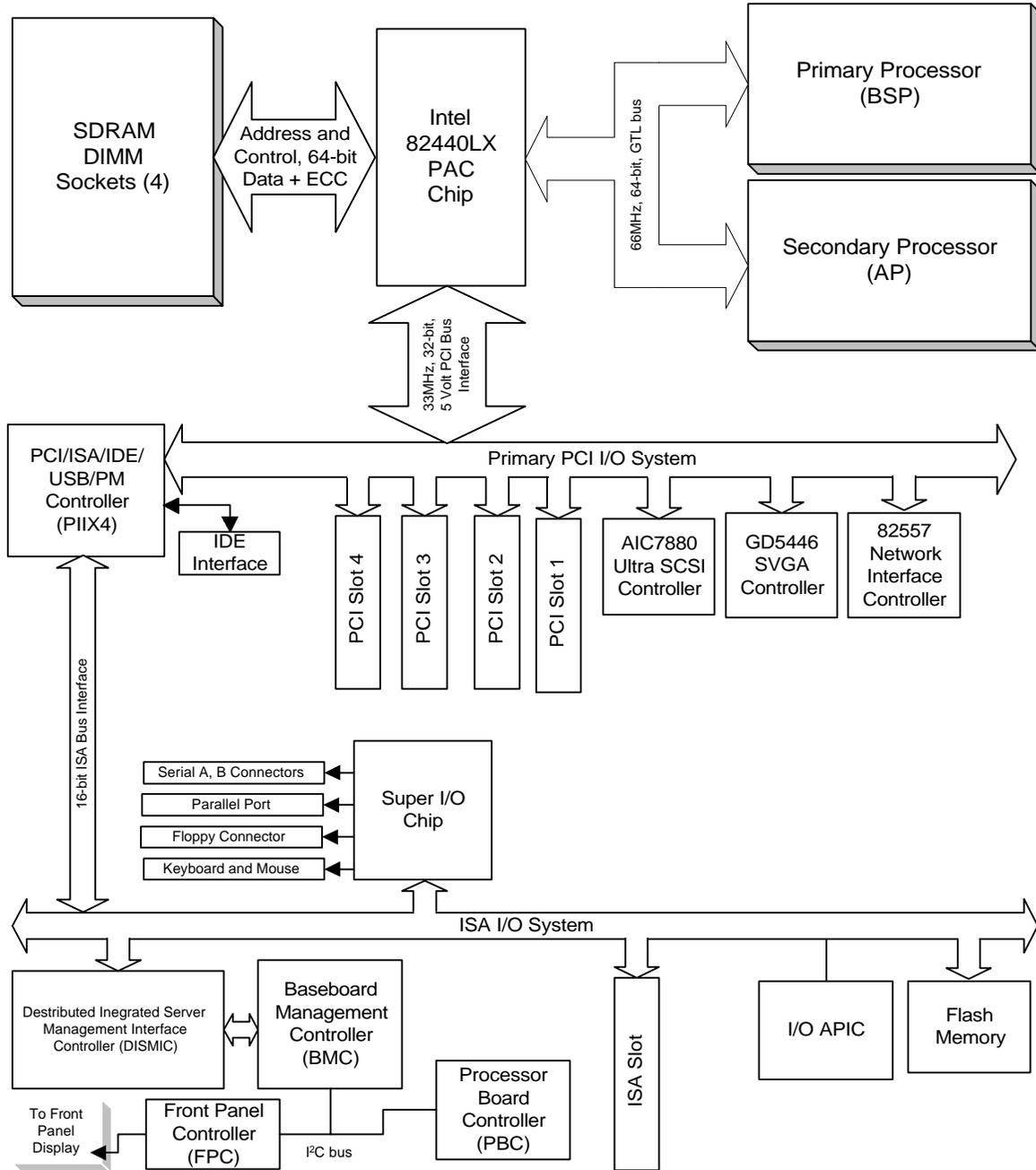
Figure 1 R440LX DP Server Functional Block Architecture
