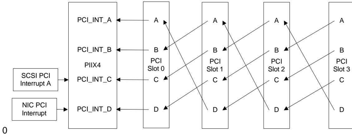
Figure 9 PCI Slot Interrupt Swizzle
