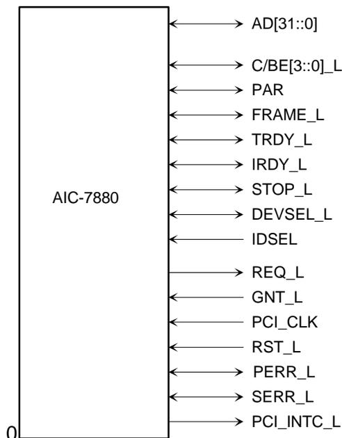
Figure 4 Embedded SCSI PCI Signals
