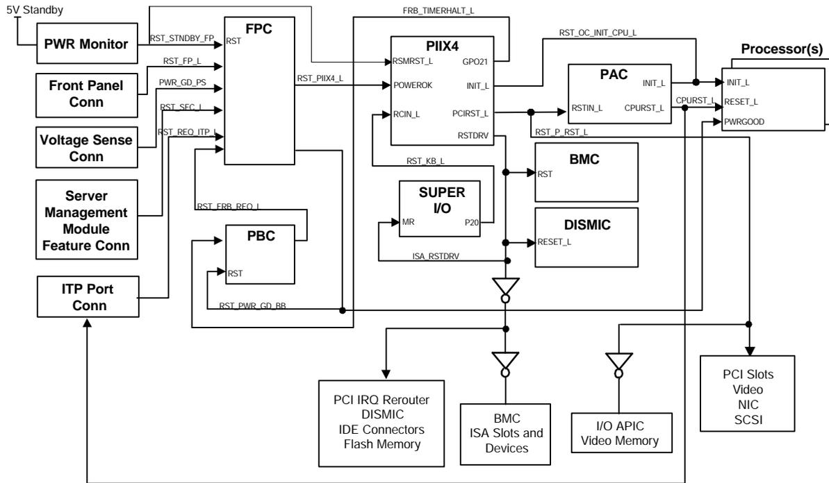
Figure 6 Reset Flow Diagram
