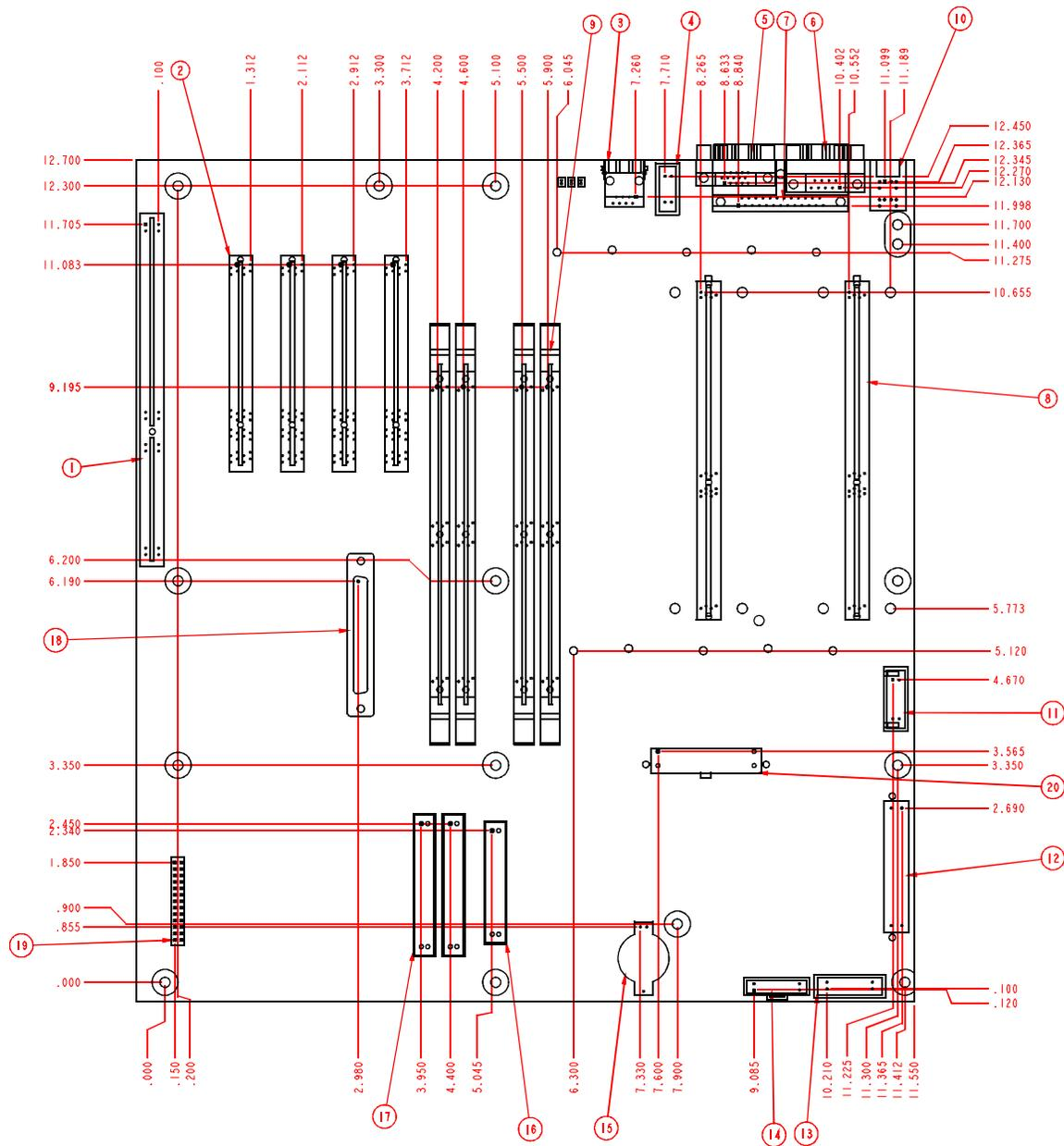
Figure 20 Baseboard Mechanical Diagram
