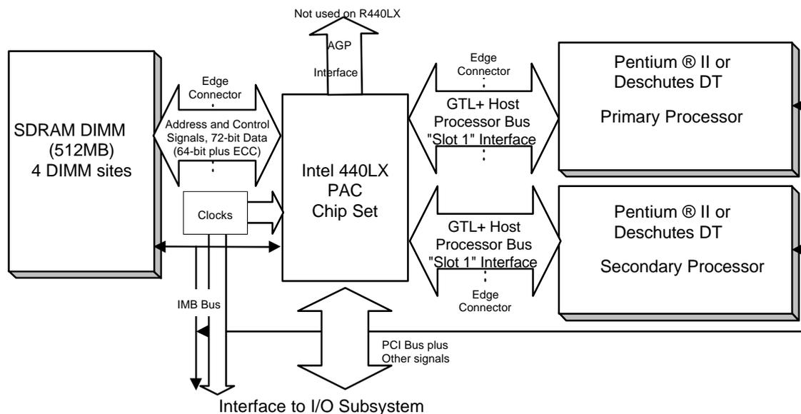
**Figure 3 Processor/PCI Host Bridge/Memory Subsystem**
