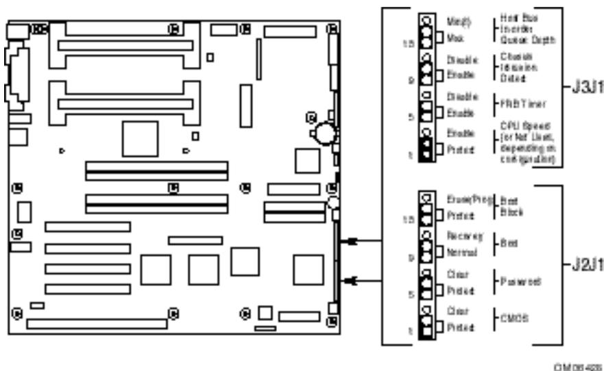
Figure 10 Board Jumper location
