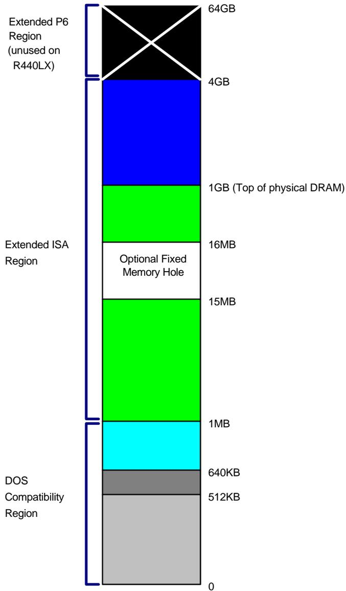
Figure 12 Pentium<sup>®</sup> II Processor Memory Address Space
