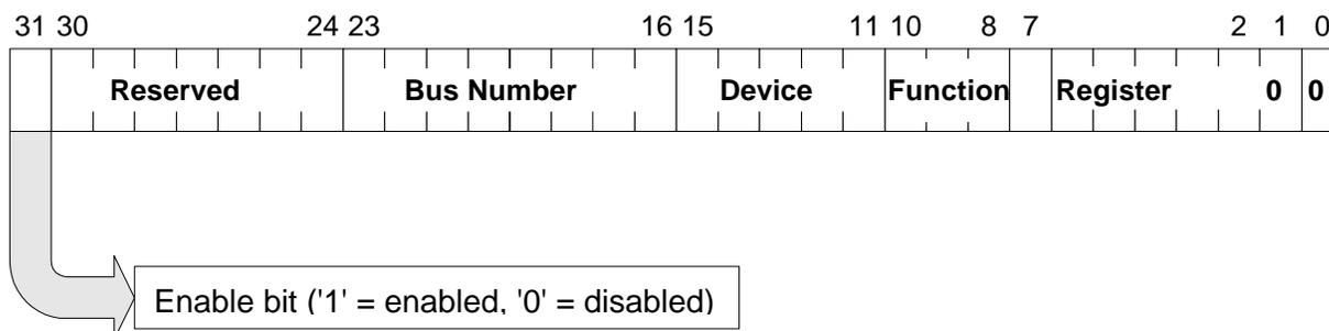
Figure 15 CONFIG\_ADDRESS Register
