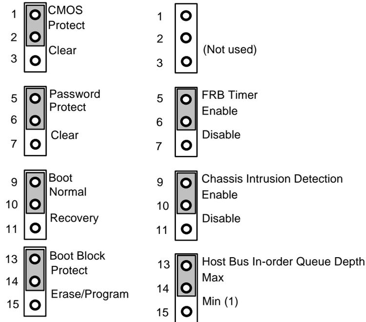
**Figure 17 System Configuration Jumpers**
