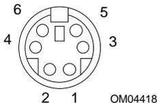
These PS/2-compatible connectors share a common housing; they are functionally equivalent.
