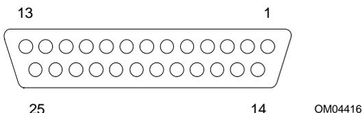
The IEEE 1284-compatible parallel port, used primarily for a printer, sends data in parallel format.
