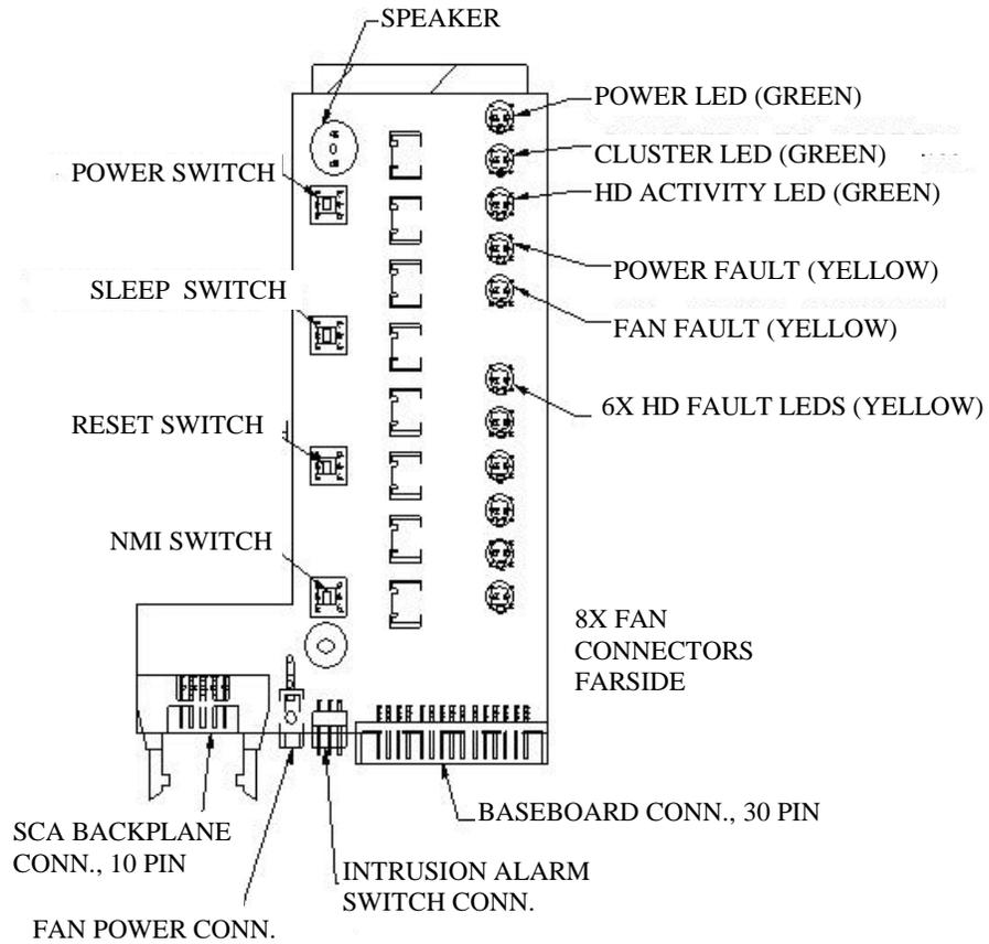
Figure 3. S450NX MP Server Front Panel
