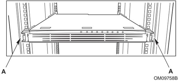
2. Slide the server out of the rack as far as you can. When the rail assembly locks, press the lock arm (A) on both sides to release the server.
