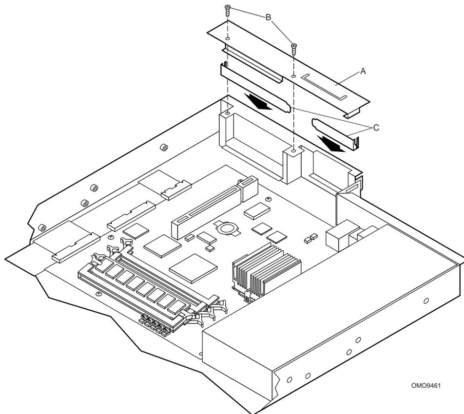
Figure 23. Installing the Rear I/O Filler Panel(s)
