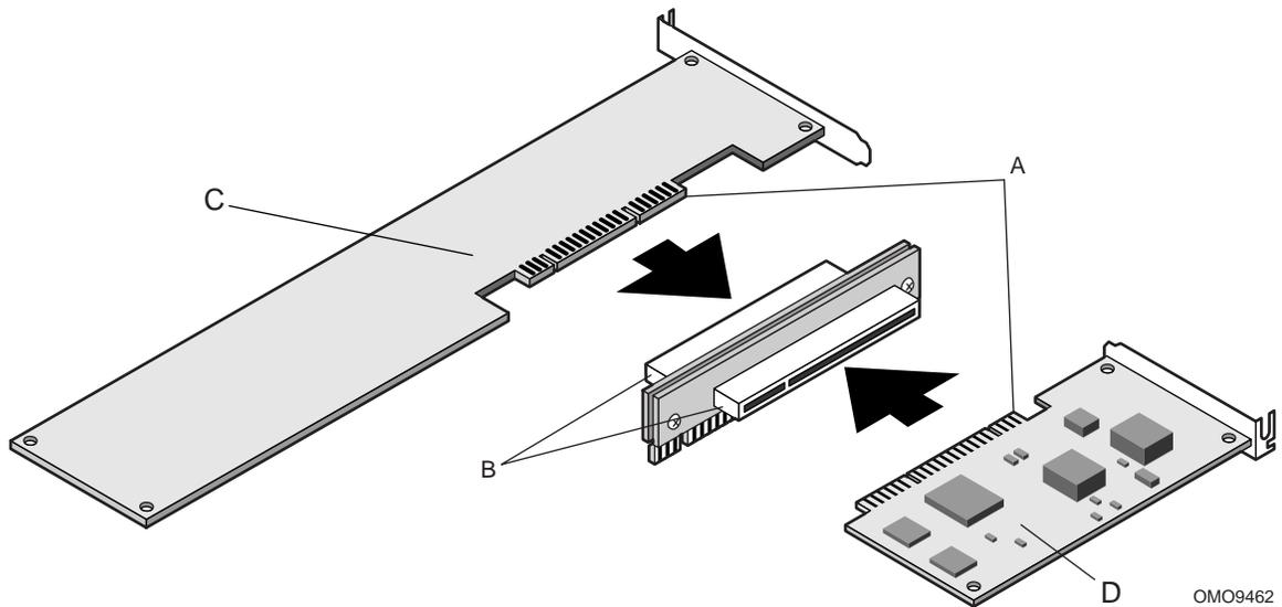
Figure 25. Installing the Add-in Card(s) on the Riser
