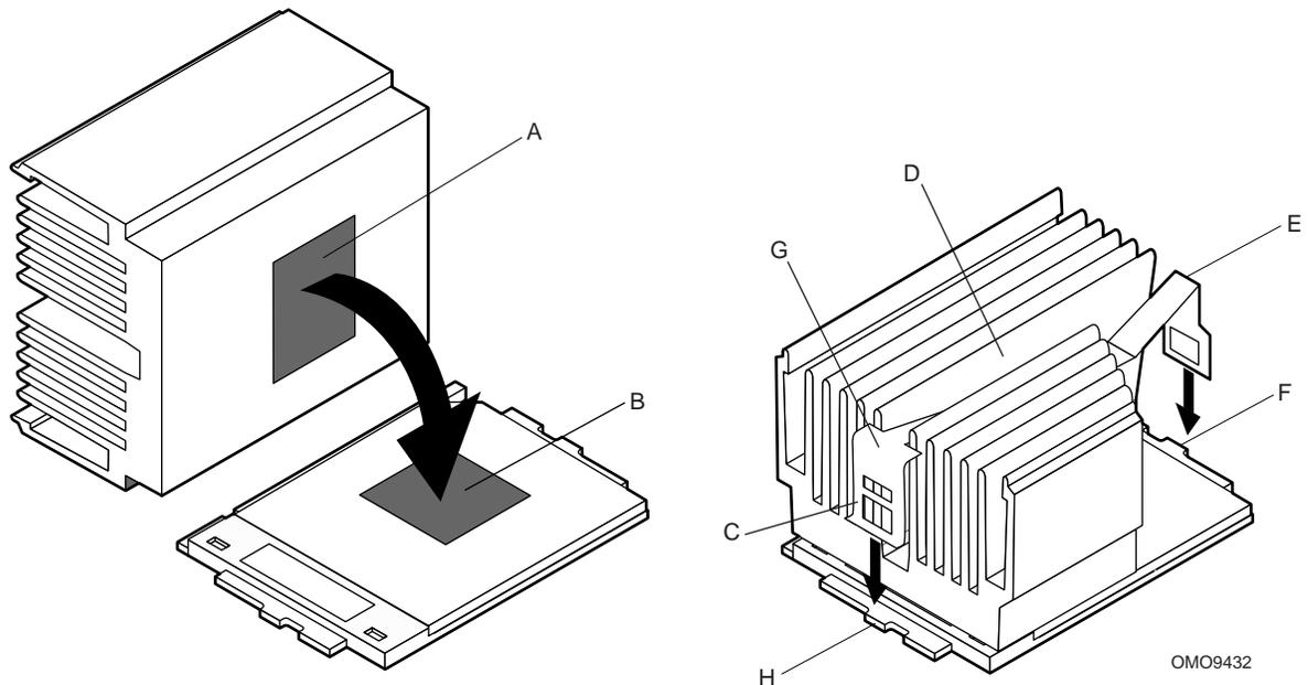
**Figure 11. Installing the Processor Heat Sink**
