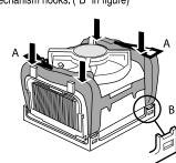
2. Firmly push the levers closed in the directions shown. It may be necessary to exert pressure to close the levers.
