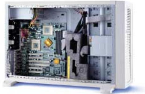
**Intel® Server Chassis SC5100** (base configuration) is designed to work with the Intel® Server Board SAI2. It includes:
