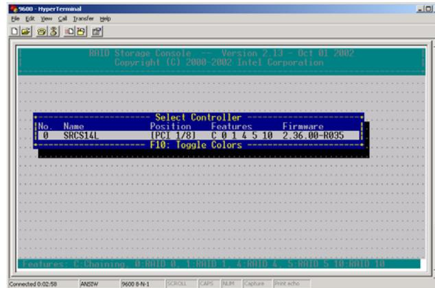
12. Press Enter to select the controller and choose the <F4> key to go to advanced options as displayed in the graphic below, then choose <C> for configure controller and <U> to update the firmware.
