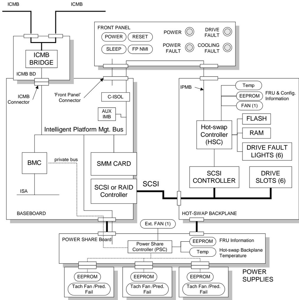
**Figure 2. Example 2, Server System Field Replaceable Unit Locations**
