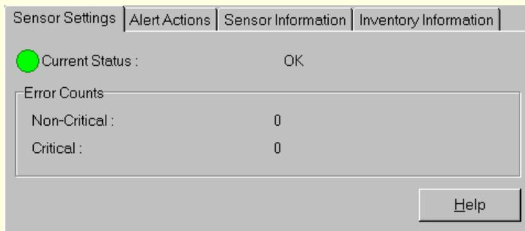
If a power supply reports a predictive failure condition, then PIC reports the status as a non-critical condition in the health branch of the PIC Console software, and the requested event actions are carried out.
