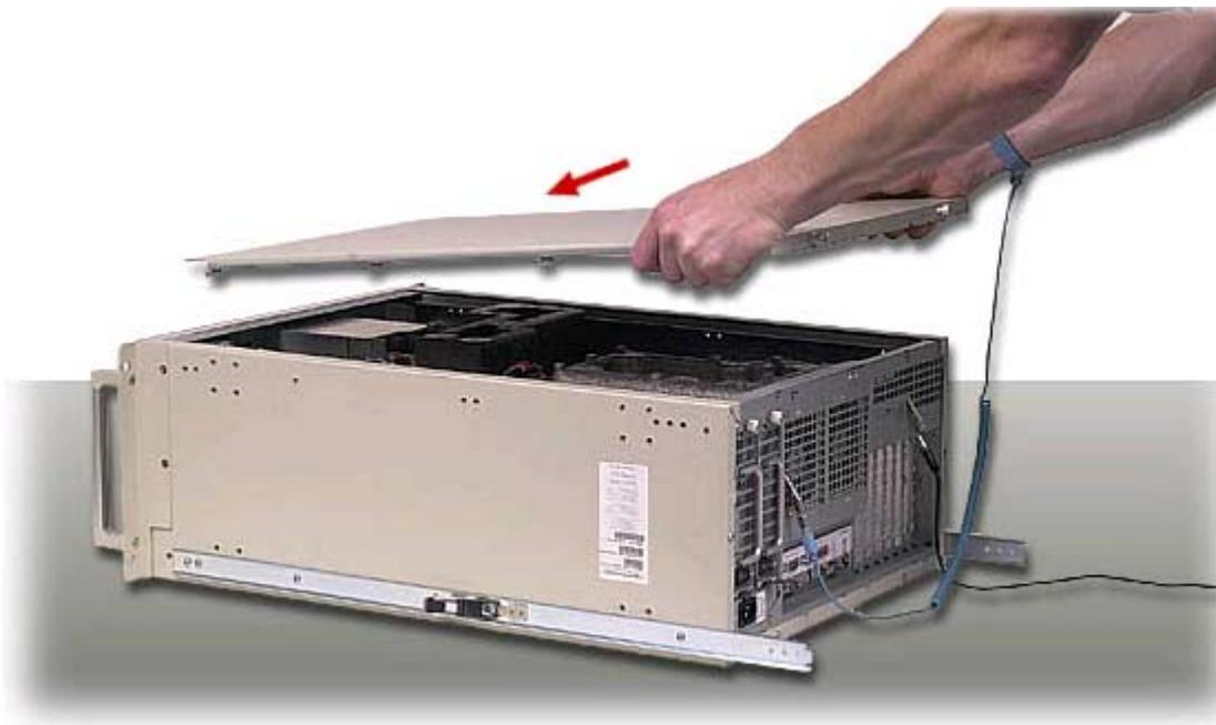
5. Holding cover at an angle, insert into chassis.
