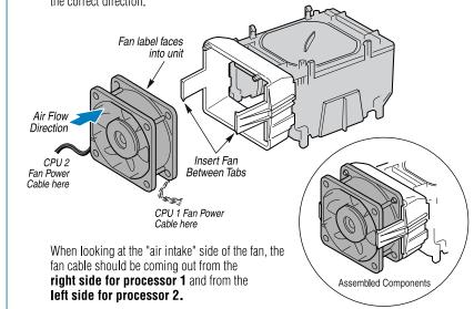
C. Attach the Wind Tunnel to the Processor Assembly
