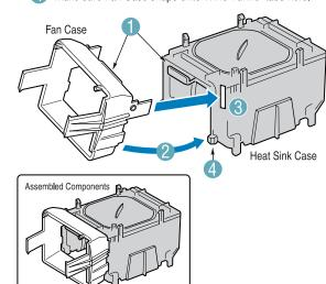
Note: Although the fan can be mounted at the top of the wind tunnel, for adequate DIMM cooling only the diagrammed installation below is recommended.
