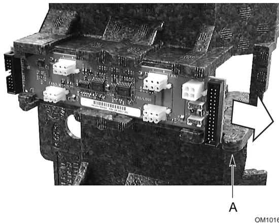
**Figure 39. Removing and Installing the Fan Distribution Board**
