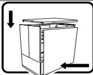
For proper cooling and airflow, always reinstall the chassis covers before turning on the system. Operating the system without the covers in place can damage system parts. To install the covers:
