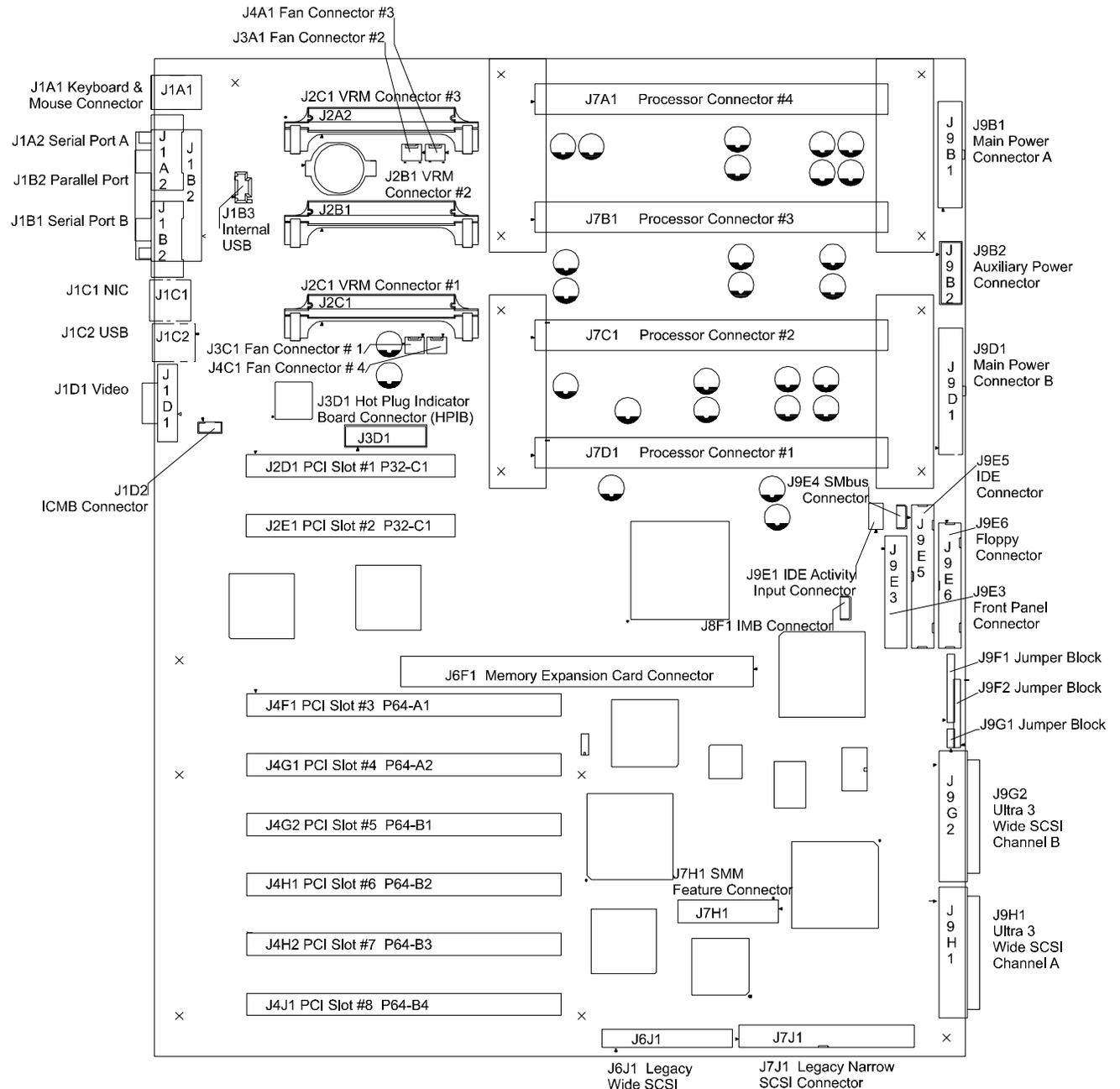
**Figure 11-1: SKA4 Baseboard Connector Identification and Locations**
