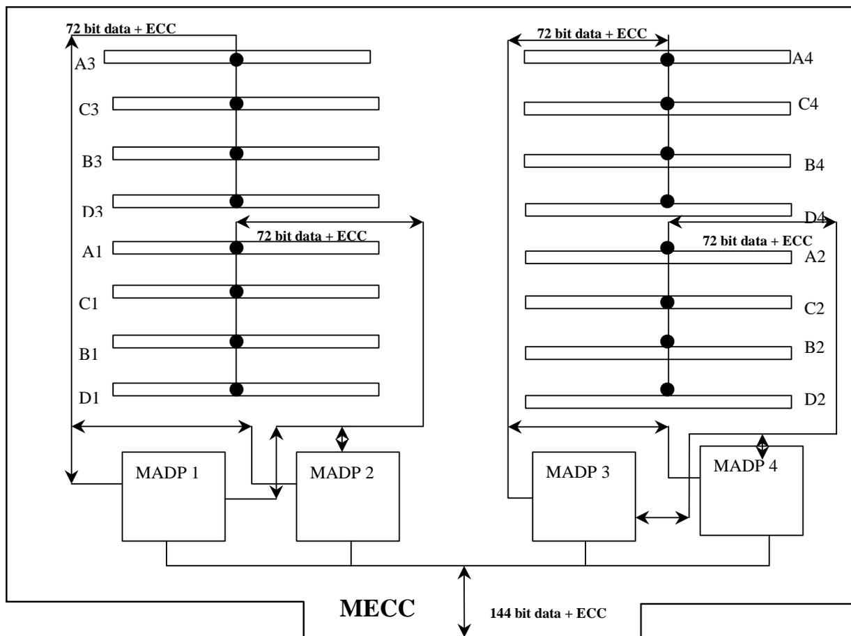
Figure 5-2: SKA4 Memory Board Functional Block Diagram
