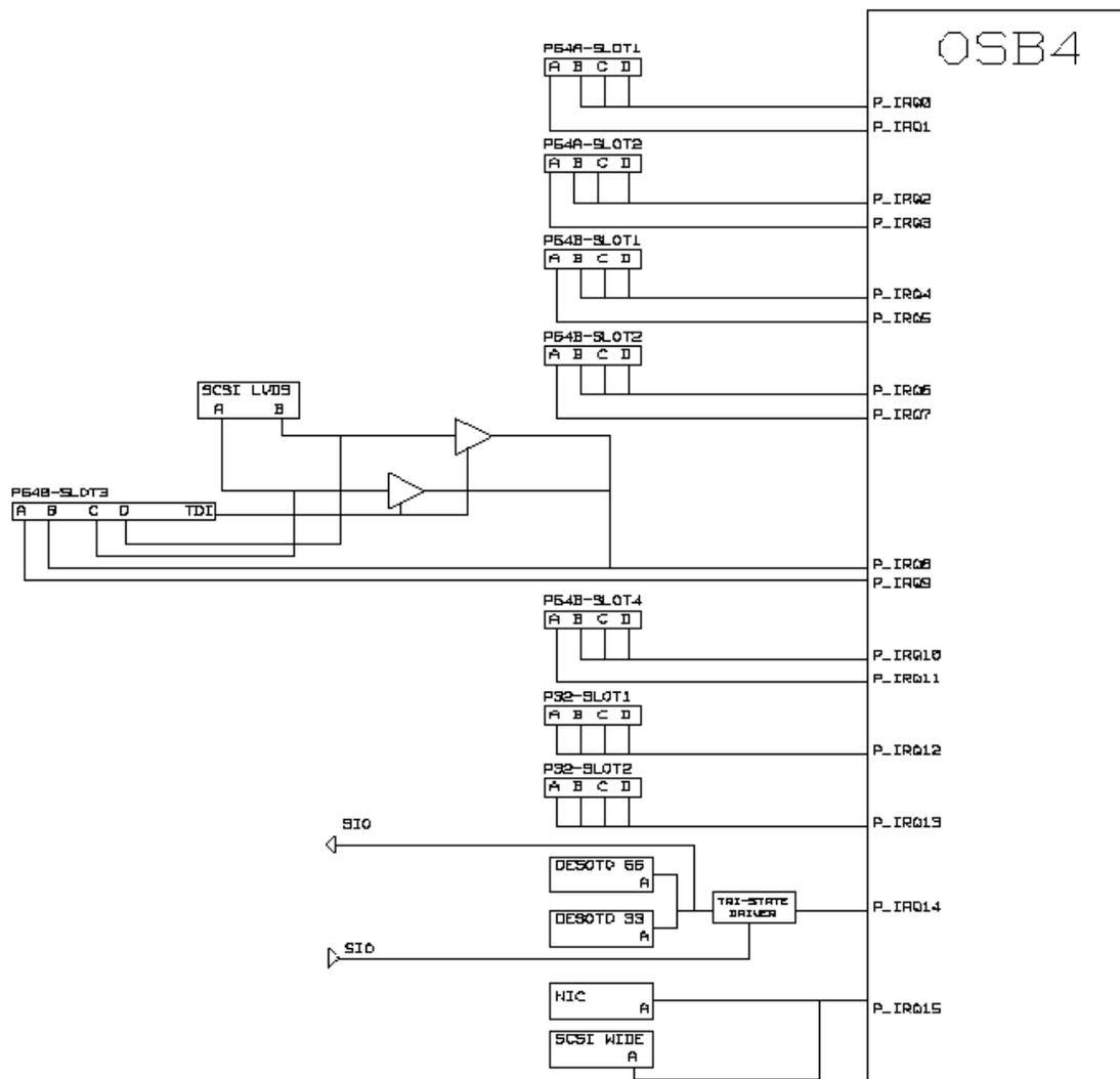
Figure 3-1: SKA4 Baseboard Interrupt Diagram
