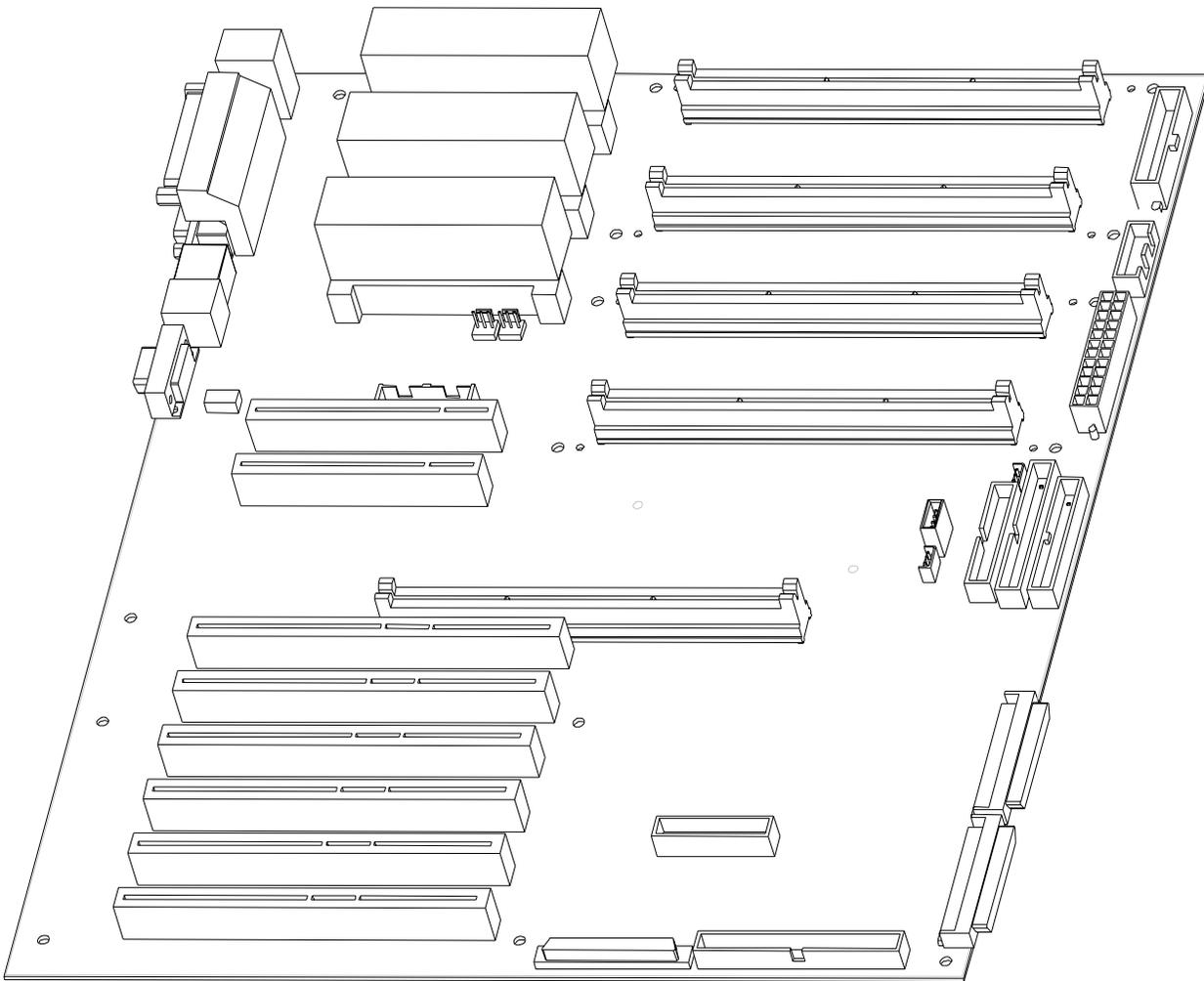
**Figure 1-2: SKA4 Baseboard Preliminary Placement Diagram**
