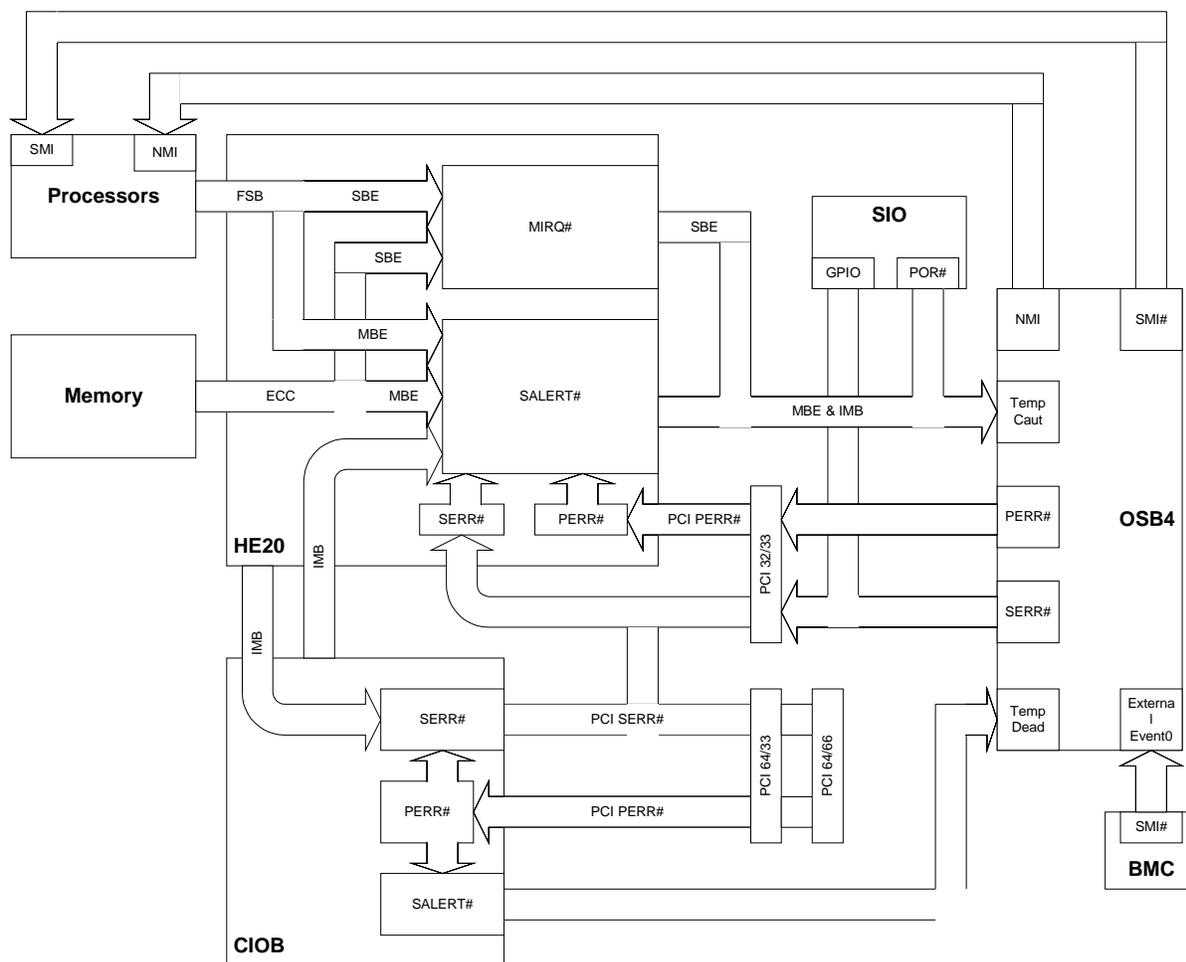
Figure 8-1: SKA4 Error Signal Propagation to SMI#
