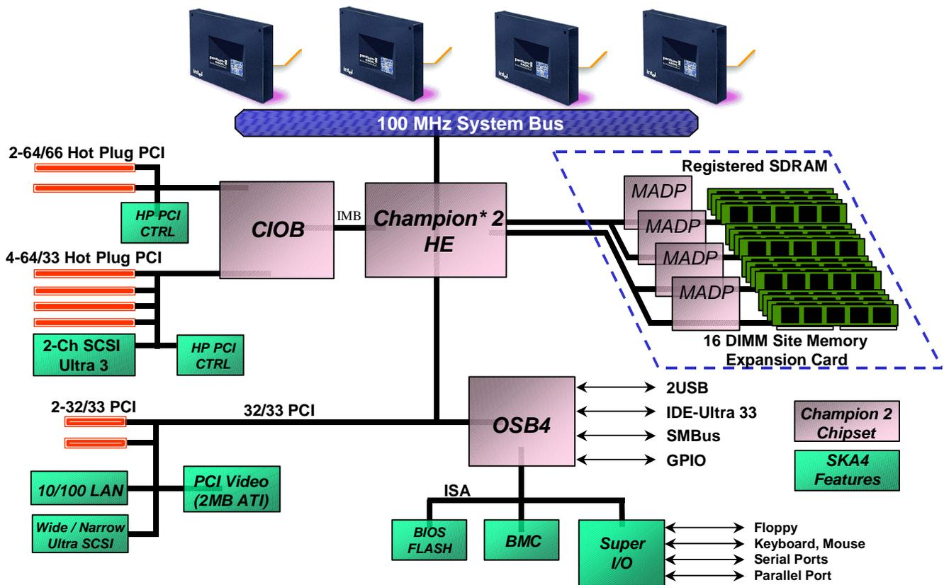
Figure 1-1: SKA4 Baseboard and MEC Block Diagram
