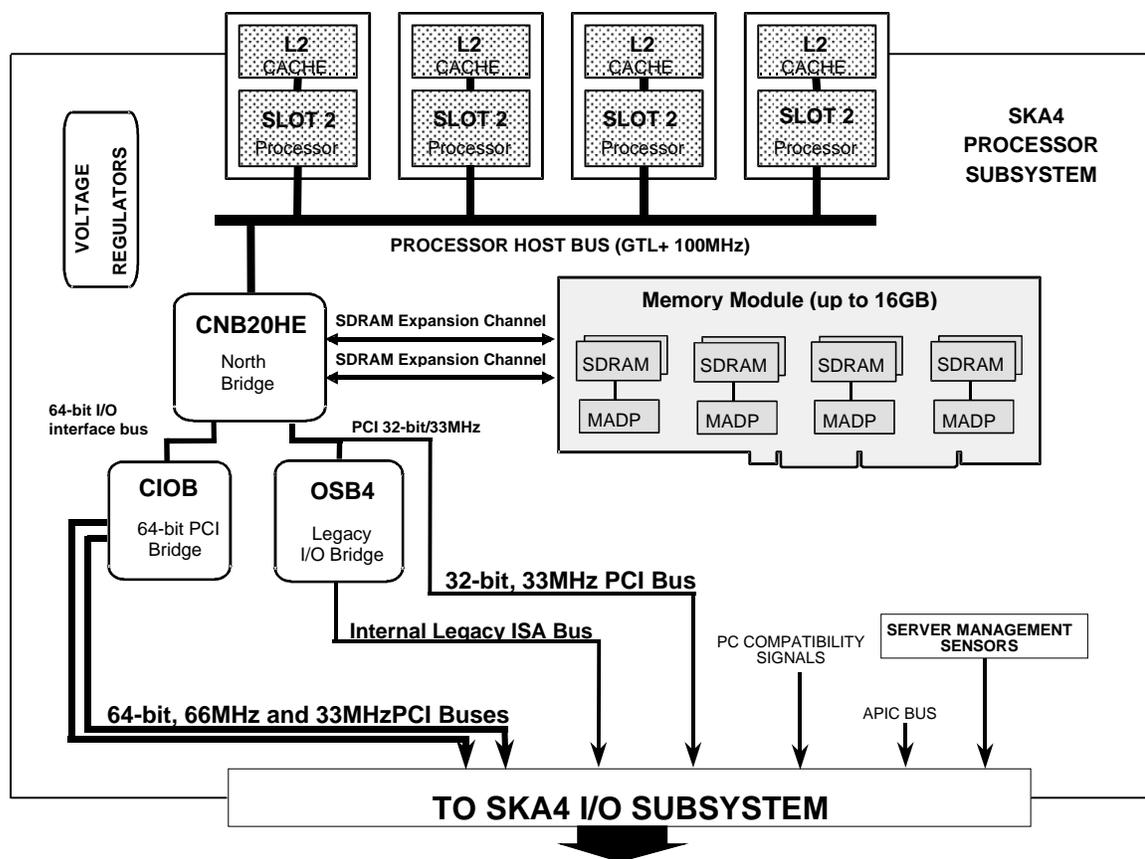
Figure 2-1: SKA4 Processor Functional Blocks
