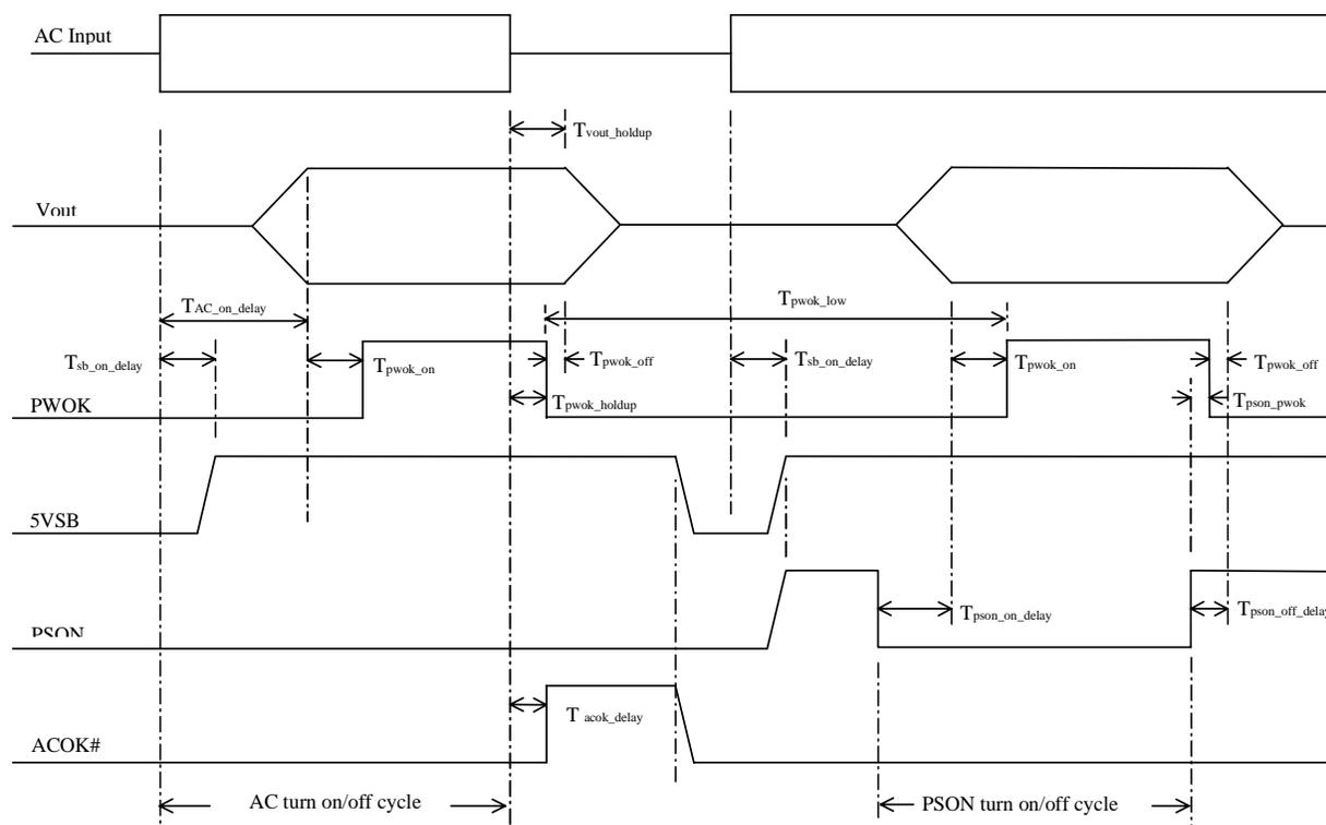
**Figure 12-2: Turn On/Off Timing**
