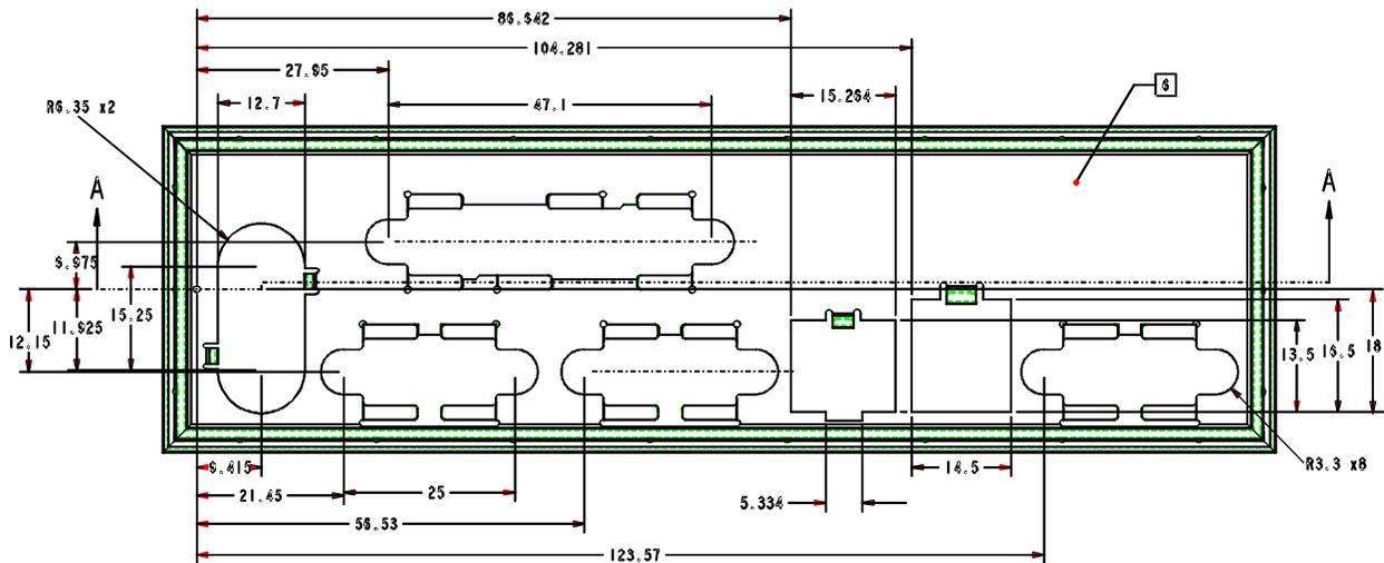
Figure 11-2: SKA4 I/O Panel Connector Location Dimensions
