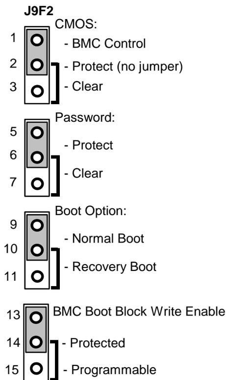
**Figure 10-1: SKA4 Configuration Jumpers**
