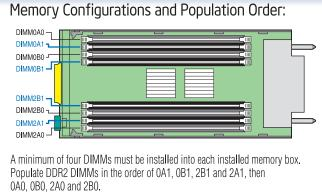
DIMMs 0A0, 0A1, 0B0, and 0B1 are positioned in reverse orientation from 2B1, 2B0, 2A1, and 2A0. Be sure to reverse the DIMMs accordingly. Make sure the notches at the center of the DIMMs line up correctly with the tabs in the center of the sockets. For additional memory information, see the Product Guide that accompanied your Intel® Server System SR9000MK4U, or go to:
