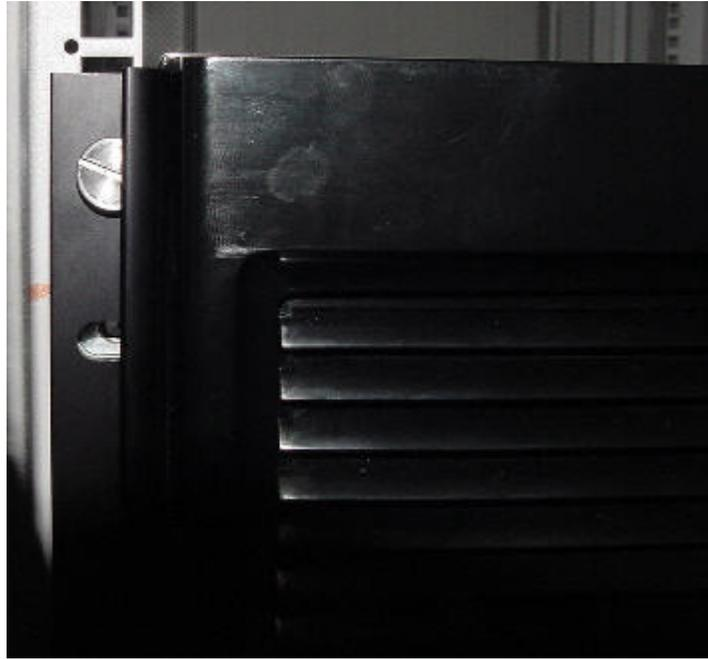
**Figure 10. Attaching the Thumbscrews, SRS4**
