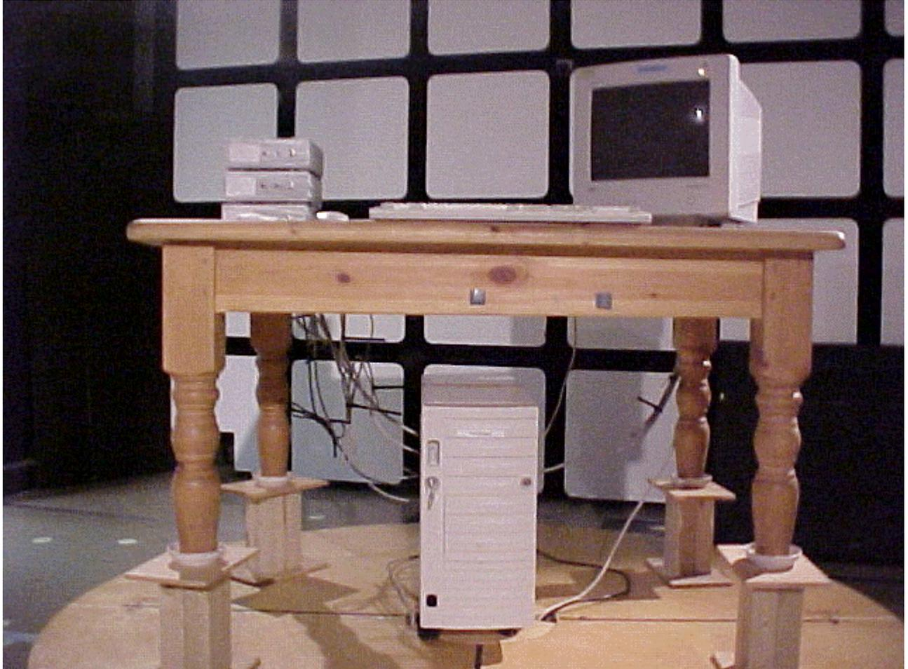
Figure 4-1 Generic test set-up
