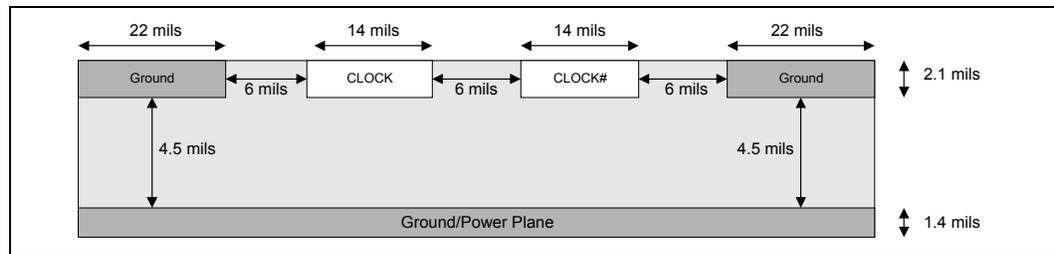
Figure 6-10. Non-Differential Clock Routing Diagram
