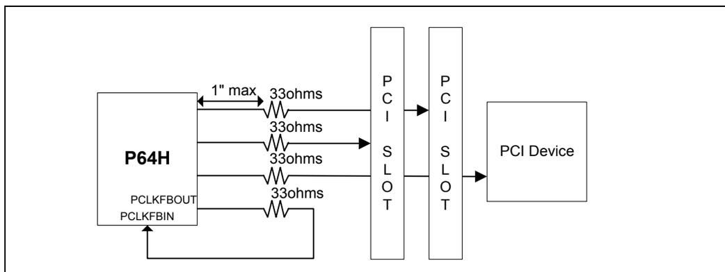
Figure 6-18. 66 MHz PCI Clock Routing
