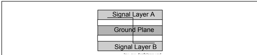
**Figure 2-4. Layer Switch with Multiple Reference Planes (same type)**
