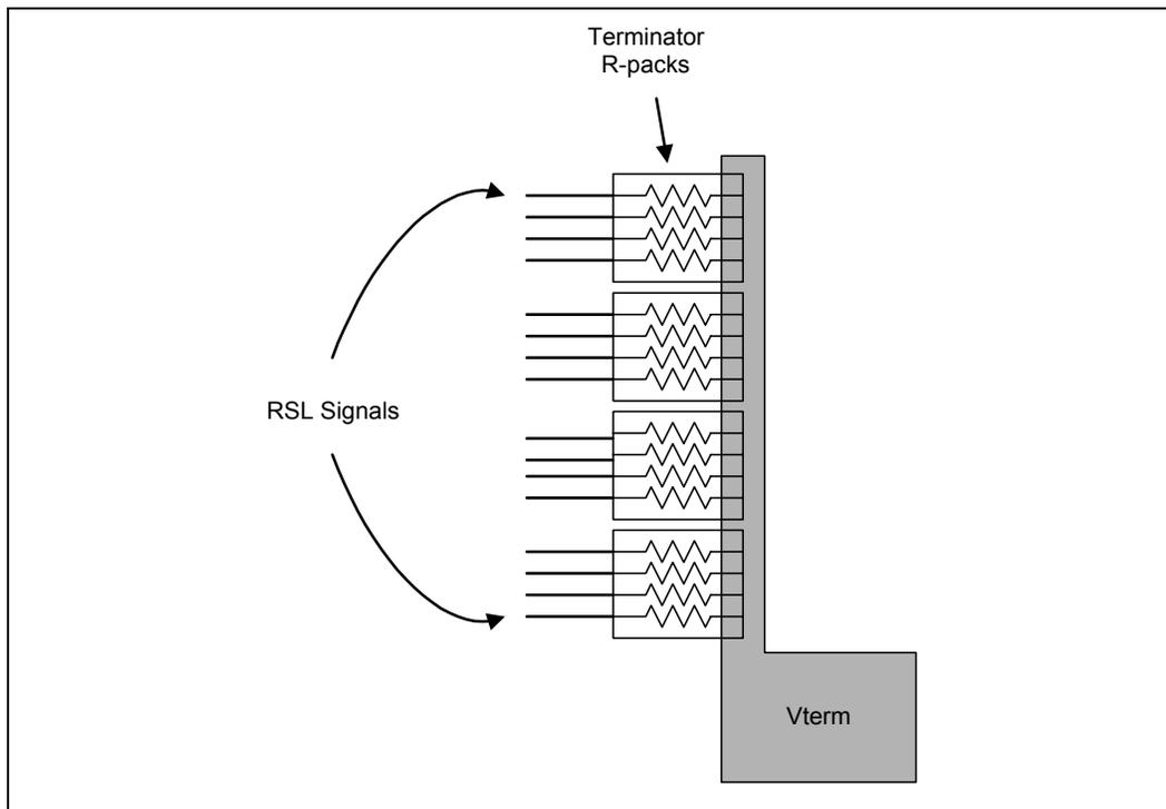
**Figure 4-14. Rambus Termination Example**
