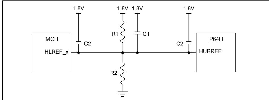
Figure 4-31. 16-Bit Hub Interface with Locally Generated Reference Divider Circuits
