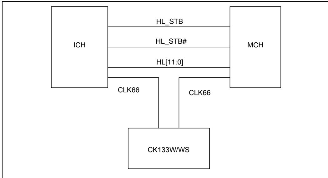
**Figure 4-27. Hub Interface B (16-Bit) Routing Example**
