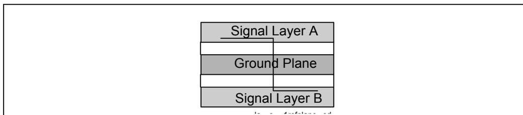
**Figure 3-4. Layer Switch with Multiple Reference Planes (same type)**
