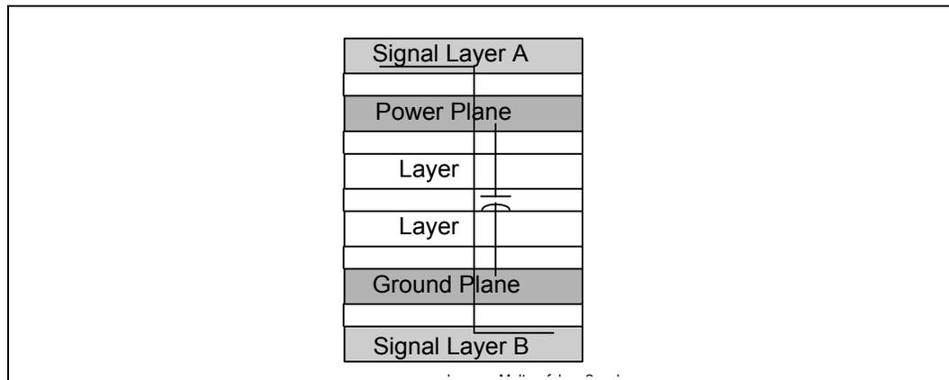
Figure 3-6. One Layer with Multiple Reference Planes
