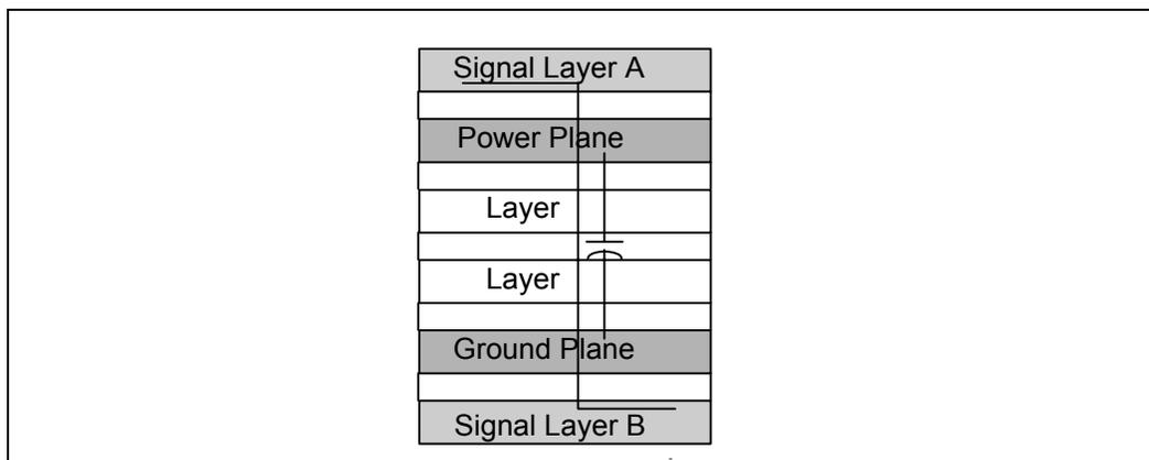
**Figure 2-6. One Layer with Multiple Reference Planes**
