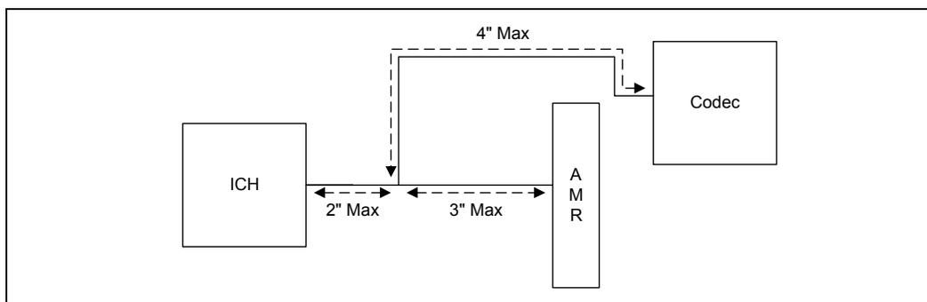
**Figure 4-38. Daisy-Chain Topology Trace Length Requirements**
