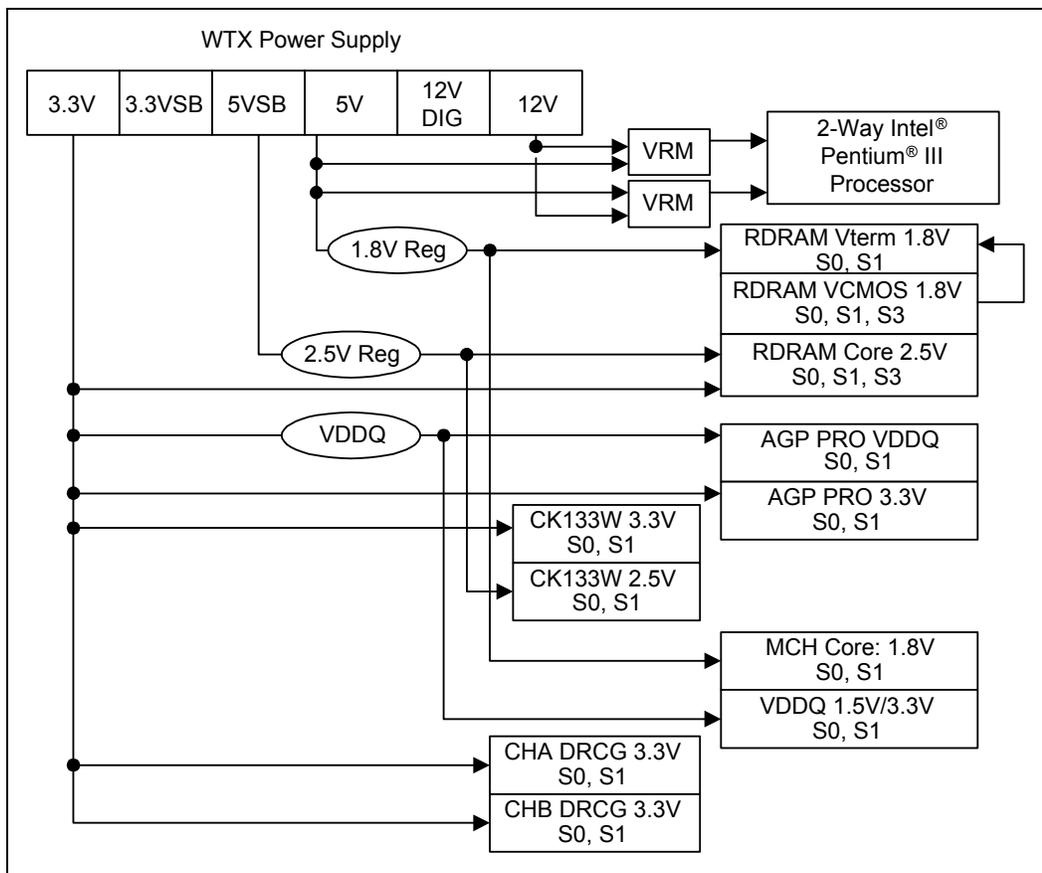
Figure 7-2. 2-Way SC242 Processors/Intel® 840 Chipset MRH-R MEC Power Delivery
