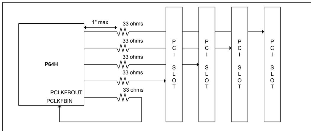
**Figure 6-16. P64H PCI 33 MHz Clock Routing**
