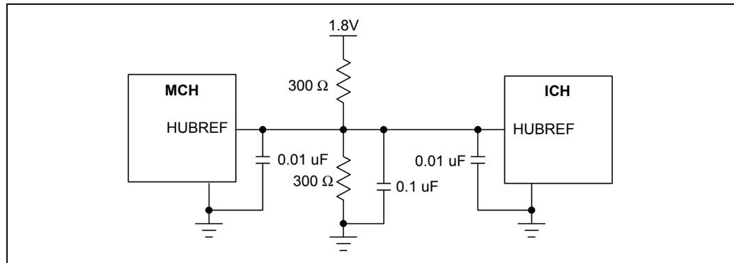
Figure 4-29. MCH/ICH Locally Generated Hub Interface Reference Divider Circuit
