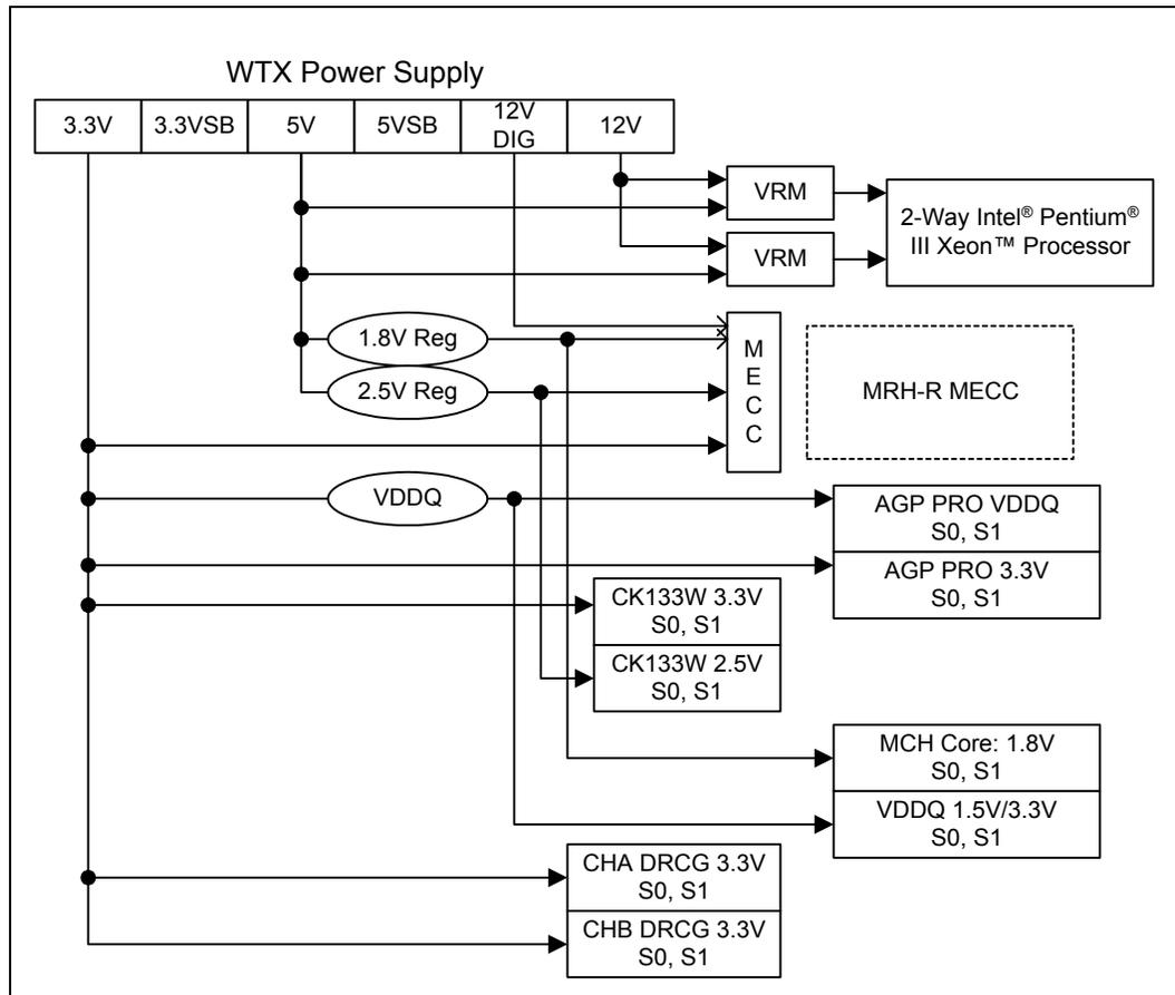
Figure 7-3. Intel® 840 Chipset System I/O Power Delivery
