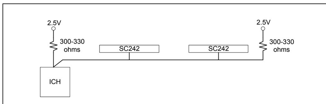
**Figure 8-3. Routing Topology Example for PICD[1:0] with P64H**
