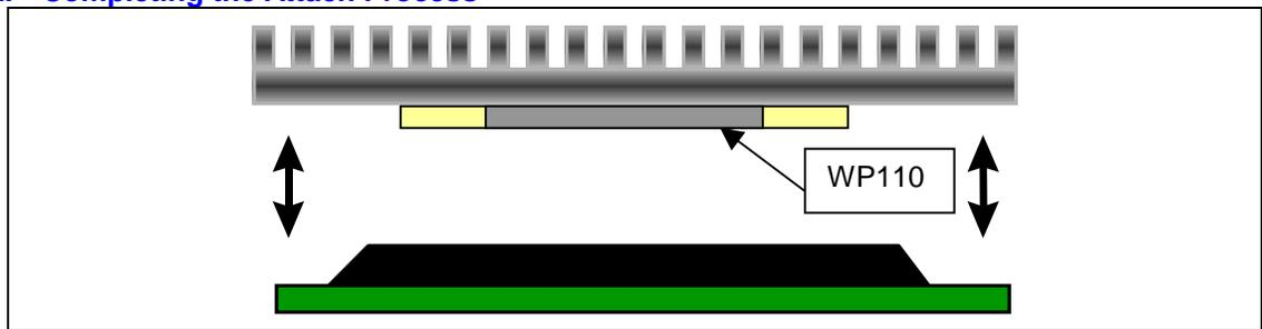
**Note:** Because each motherboard-system-heat sink combination may introduce variation in the attach strength, it is generally recommended that the user carefully evaluate the reliability of tape attaches prior to their high-volume use.
