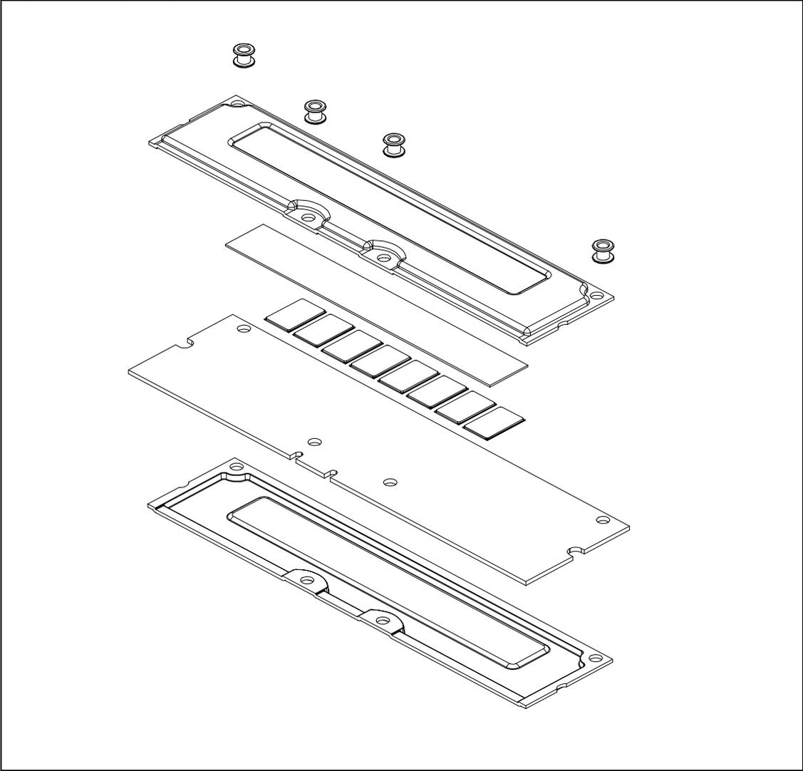
Figure 6. Mechanical Drawing (Reference RIMM)
