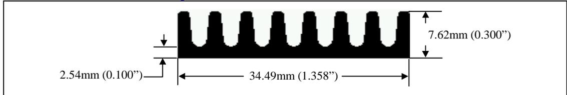
Figure 10. Extruded Heat Sink Drawing for the P64H
