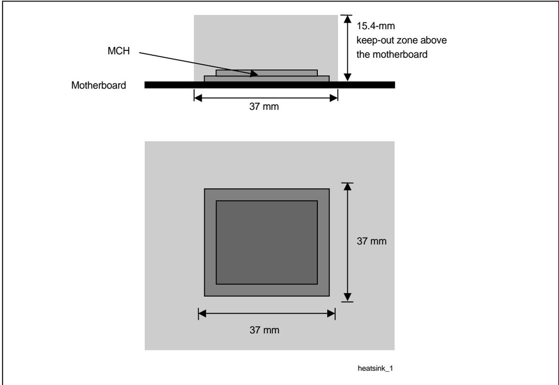
Figure 8. Heat Sink Volume Restrictions for the P64 When Attached to the Motherboard
