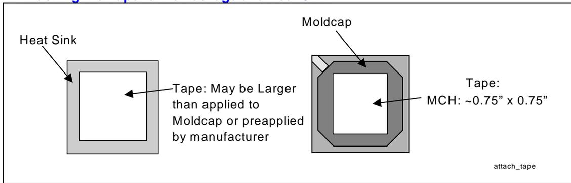
**Figure 15. Completing the Attach Process**
