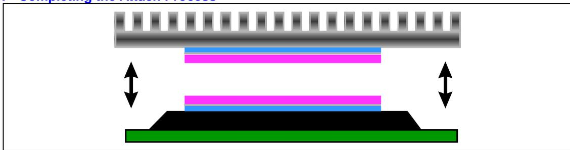
**Note:** The silicone adhesive always joins to either the heat sink or the mold-cap. The acrylic adhesive sides must join to each other (Figure 15)
