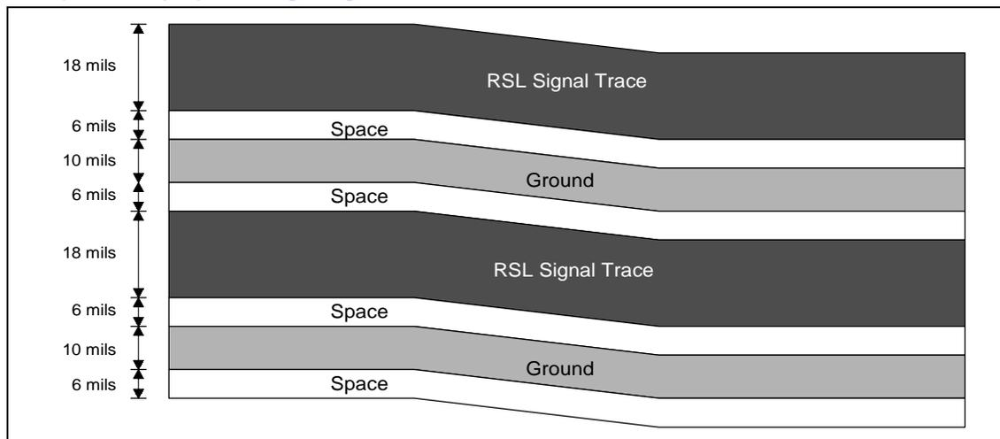
Figure 5 shows a top view of the trace width/spacing requirements for the RSL signals when routing on outer layers.
