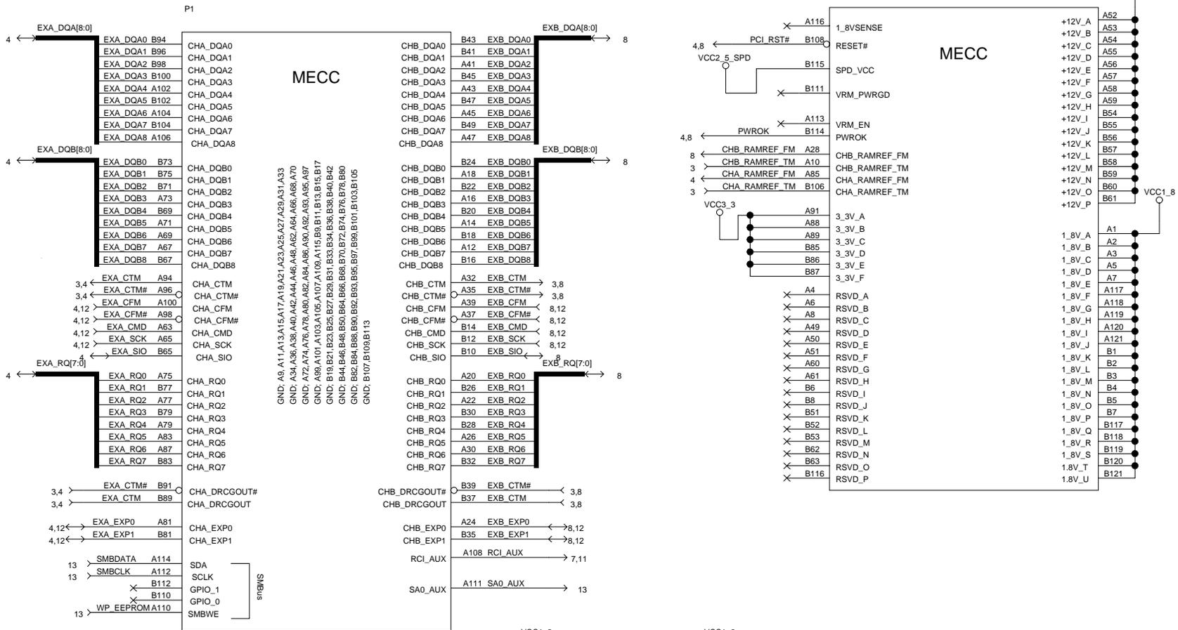
GND: A9, A11, A13, A15, A17, A19, A21, A23, A25, A27, A29, A31, A33
