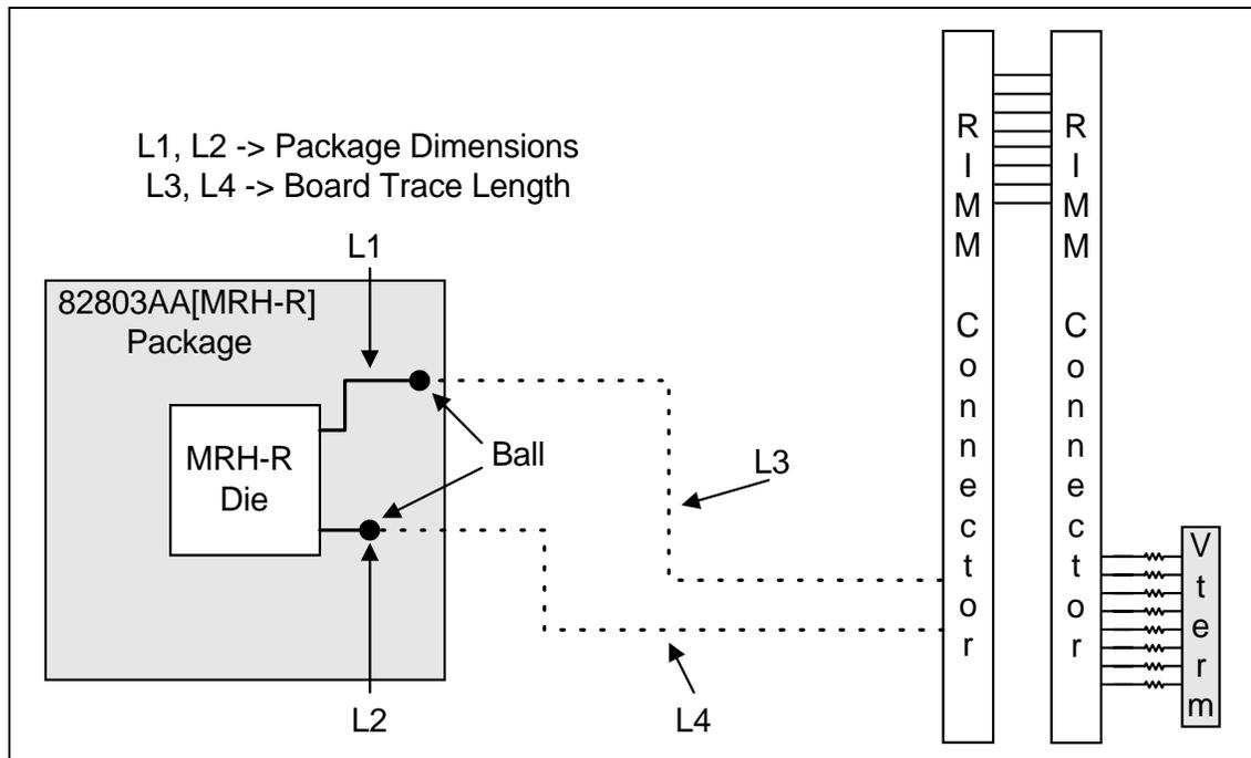
**Figure 11. RDRAM Trace Length Matching Example From MCH to MRH-R**
