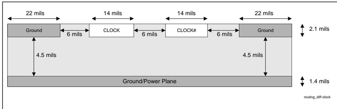
**Note:** “CLOCK” stands for the signals CTM and CFM and “CLOCK#” stands for the signals CTM# and CFM#.
