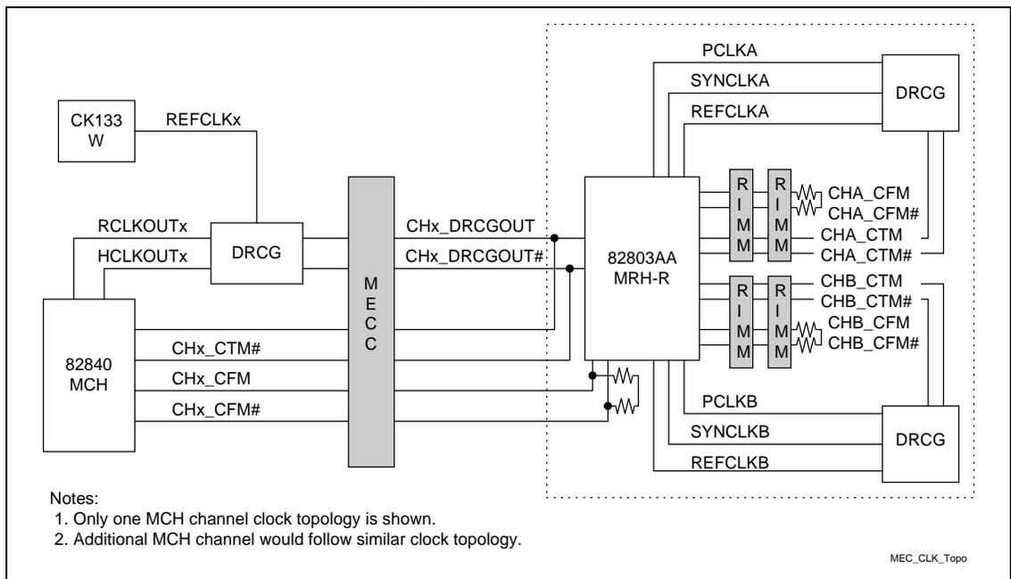
Figure 26. Additional RDRAM Clock Routing Guidelines
