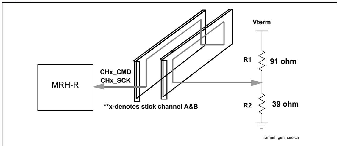
Figure 16. High-speed CMOS Termination from MCH to MRH-R
