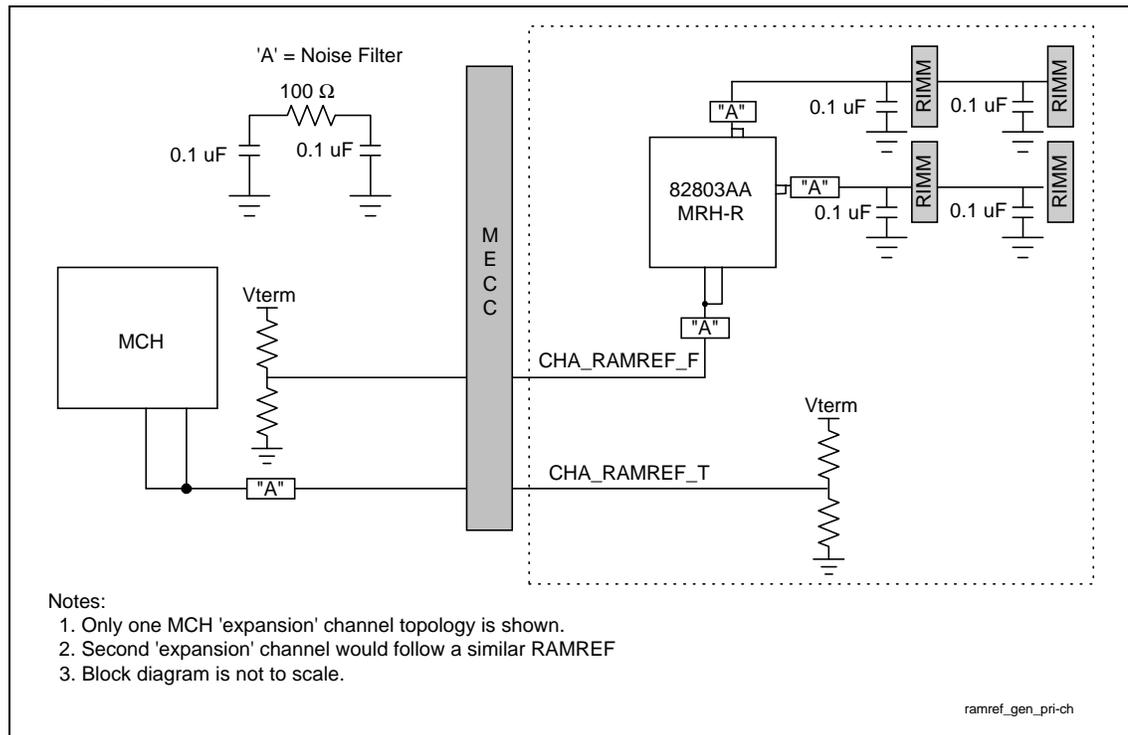
The generation of RAMREF on 'expansion' channels is different. To account for potential differences between RAMREF and GND on the motherboard and on the memory expansion cards, it is recommended using *source generated RAMREF* for the expansion channels.
