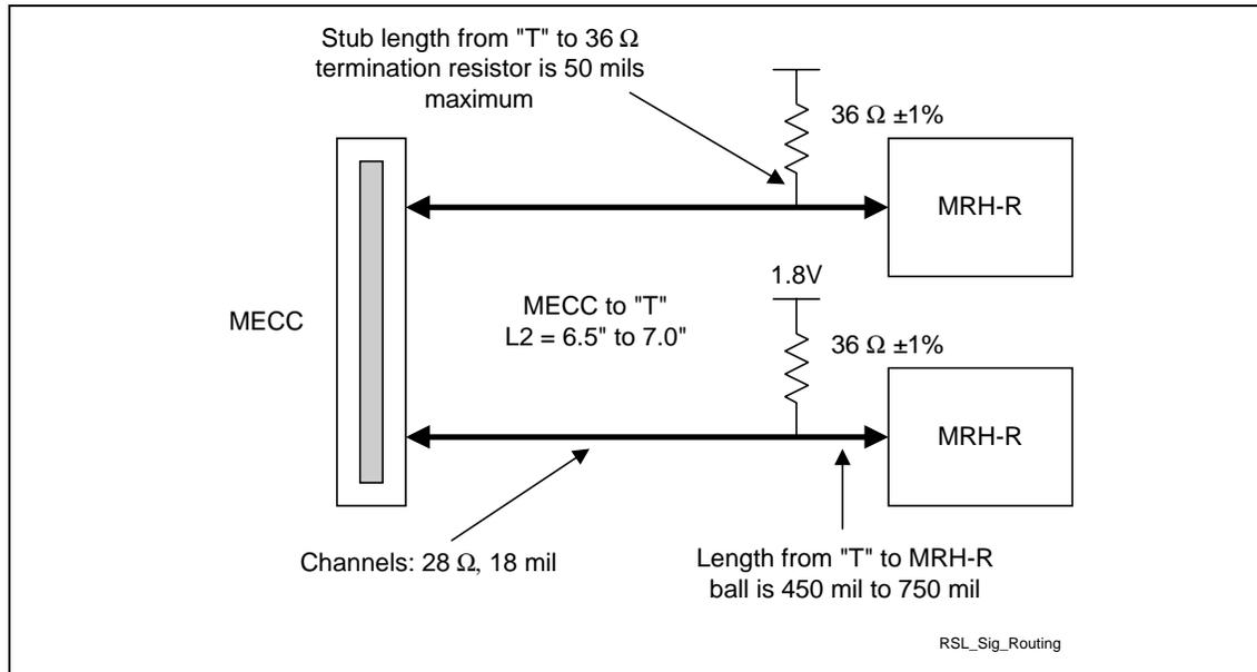
**Figure 5. RSL (Outer Layer) Routing Diagram**
