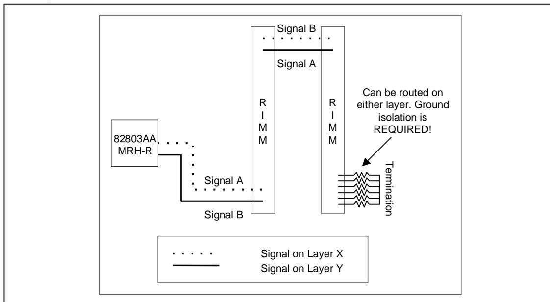
NOTE: Signals can be routed on either layer from the last RIMM to the termination resistors.
