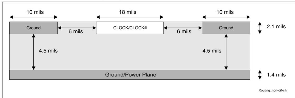
**Note:** “CLOCK” stands for the signals CTM, CTM#, CFM and CFM#.
