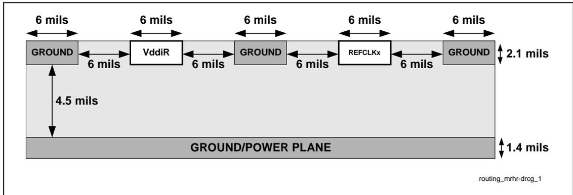
**VddIPD, PCLKM and SYNCLKN Routing Example**
