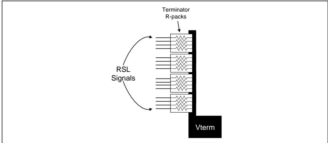
Figure 9. Direct RDRAM Termination Example
