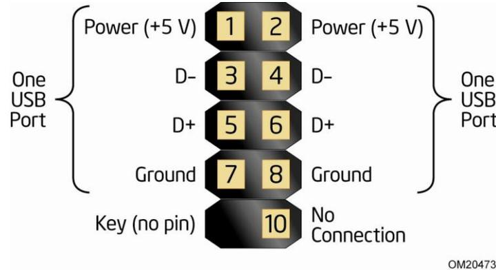
**Figure 12. Connection Diagram for Front Panel USB Headers**
