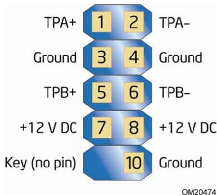
**Figure 13. Connection Diagram for IEEE 1394a Header**
