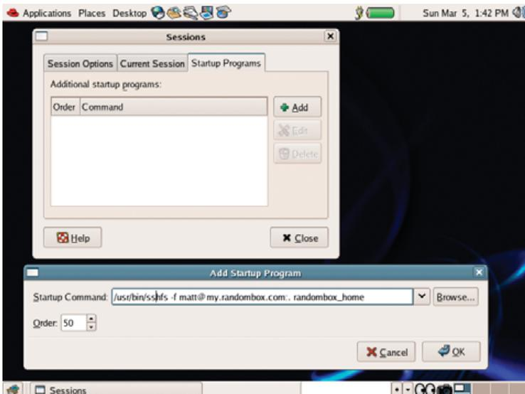
Figure 1. Set up a GNOME startup command to mount an SSHFS share.
