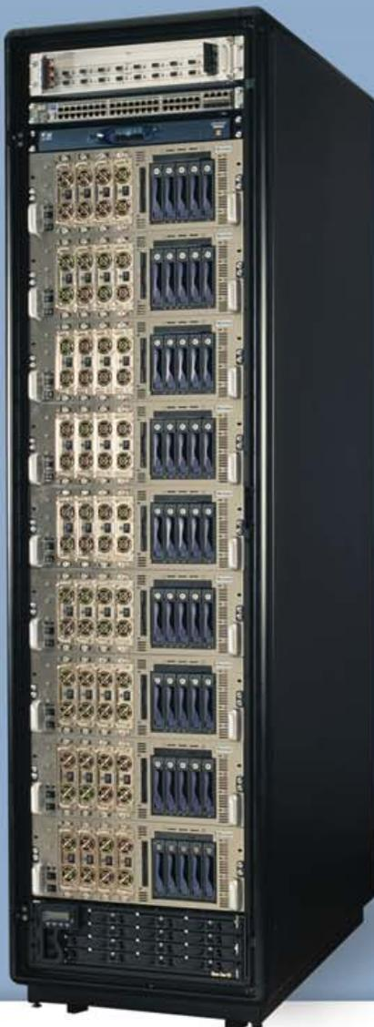
▲ Microway® Quad Opreton™ Cluster with 36 Opreton 880s, redundant power, 45 hard drives and Myrinet™ in our CoolRak™ cabinet.
