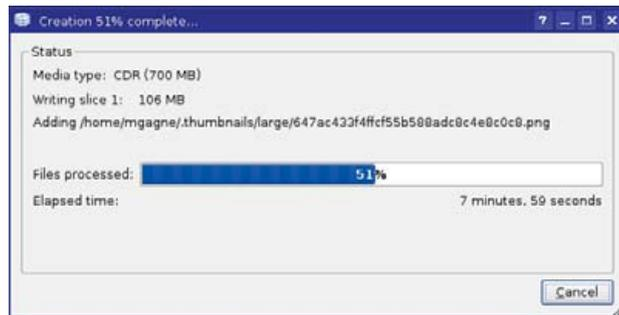
Figure 6. KDar's backups provide a graphical progress report with estimated time to completion.
