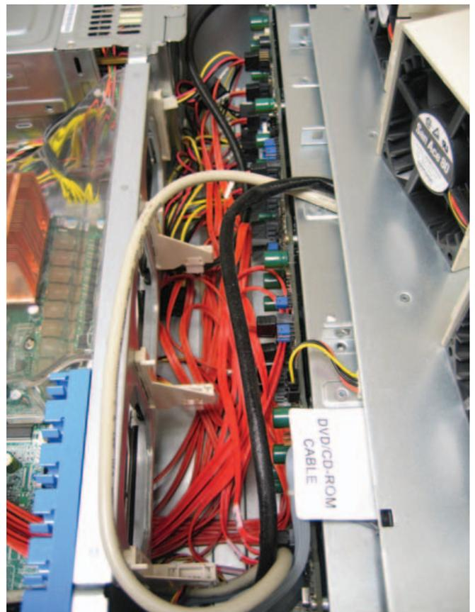
Figure 3. SATA Backplane with Cooling Fans Removed
