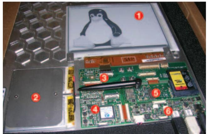
Figure 3. Picture and Block Diagram of the Hardware: 1 E-Ink Vizplex Display, 2 Li Ion Battery, 3 Display Adapter Board, 4 Metronome Display Controller Board, 5 Gumstix Board and 6 Lyre Mainboard
