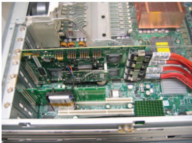
Figure 4. 3ware RAID Controller with Remote Battery Option
