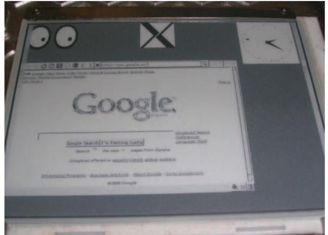
Figure 2. Running Dillo, xeyes, XClock and XLogo on an E-Ink Display
