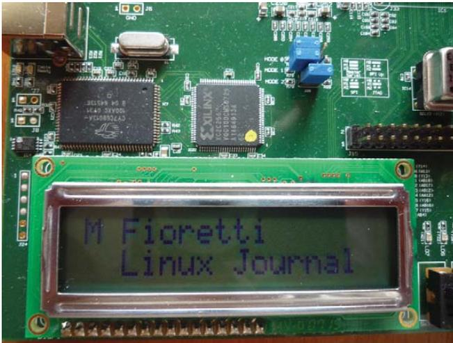
Figure 9. Program Running on FPGA Hardware
