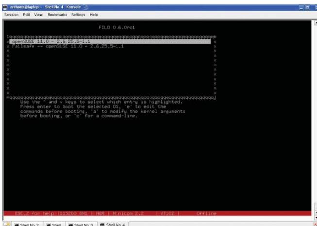
Figure 2. You can control the booting process via minicom.
