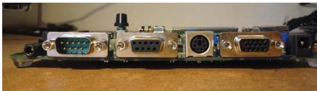
Figure 4. Stereo Mini-Jack, Serial M, Serial F, Keyboard, VGA, Power (Ethernet/USB on Other Edge)
