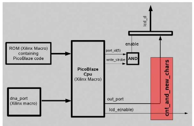
Figure 6. Simplified Circuit Diagram of the DNA Reader
