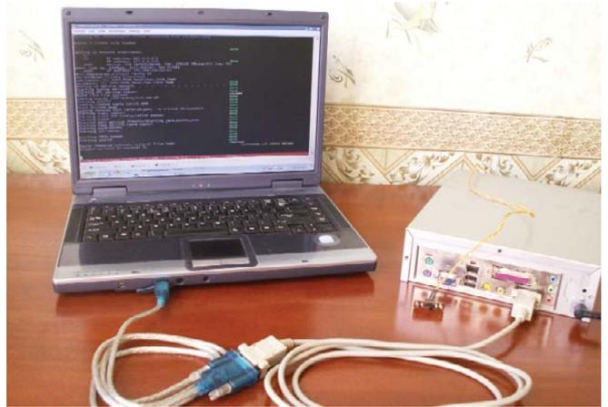
Figure 3. The operating system writes to serial port.
