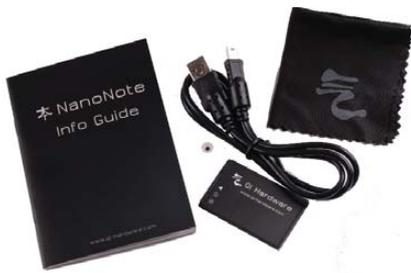
Figure 2. Included with the Ben NanoNote are a cleaning cloth, a manual, a USB cable, a battery and a little rubber nub.
