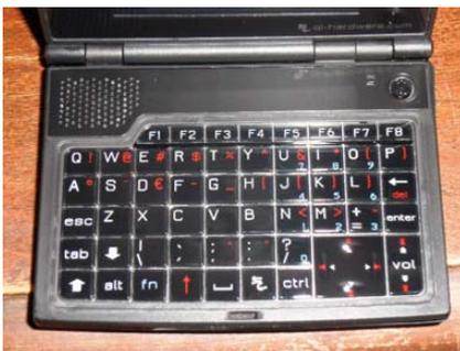
Figure 4. The Ben NanoNote's keyboard, featuring the world's smallest spacebar.
